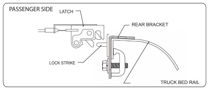
It may be necessary to adjust the latch side to side, to do so loosen the two latch mounting bolts, adjust latch and tighten.
