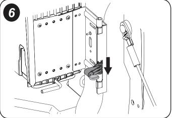
6. INSTALL THE PIVOT LOCK (figure 6) - Once the pivot lock is over the top of the lower pivot bushing, slide the pivot lock down against the top of the pivot bushing.
