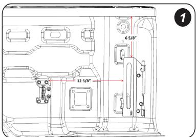
2. INSTALL THE TRUCK BRACKET AND STRIKER BRACKET (figure 2) - Install the truck bracket and striker bracket using the provided self drilling screws - four for each bracket. Use a 7/16" wrench or socket and tighten to 10 +- 1.0 Nm. Be careful not to overtighten and stripe out the holes.
