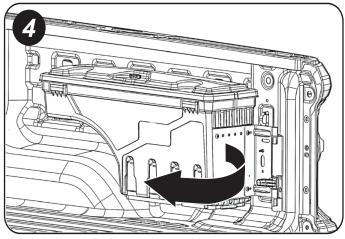
4. CLOSE AND LATCH THE SWINGCASE (figure 4) - Swing the Swingcase to the truck bed wall to latch it in place.
