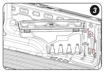
3. INSTALL THE SWINGCASE (figure 3) - Lift the case, align the openings of the case bracket to the pins of the truck bracket and lower the Swingcase onto the pins.
