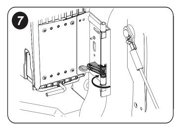
7. INSTALL THE PIVOT LOCK (figure 7) - Rotate the pivot lock towards the box bracket, so that the pivot lock is against the bracket and lines up with the slotted hole in the bracket.
