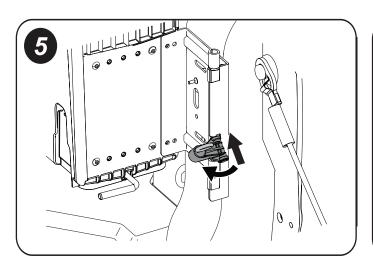
5. INSTALL THE PIVOT LOCK (figure 5) - Insert the supplied pivot lock at an angle between the lower tab and the top of the lower pivot bushing. While pushing upward on the pivot lock, rotate the pivot lock into position over the top of the lower pivot bushing.
