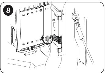
8. INSTALL THE PIVOT LOCK (figure 8) - Rotate the key 90 degrees into the locked position.
