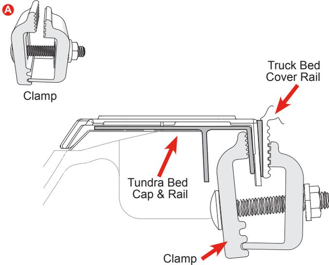
Position the driver side rail against the truck's bed rail. Begin clamping the driver side rail to the truck bed. Start in the middle and evenly space 3 clamps (A) along the rail. You should leave approximately 8" on each end of the rail. Finger tighten the clamps, making sure the teeth properly engage with the grooves of the side rail. Repeat on the passenger side rail.
