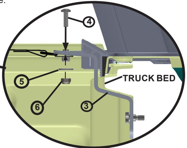
**STEP 4:** With everything loosely assembled tighten all six M6 Shoulder bolts making the bracket tight to the truck bed, leaving the rails able to move.
