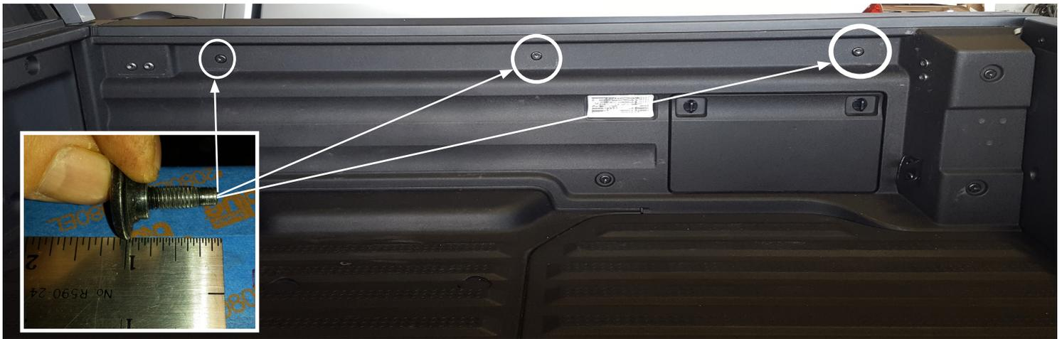
**STEP 2:** Mount brackets on driver and passenger sides using the factory installed M6 Shoulder bolts. Do not fully tighten these bolts, just tighten them finger tight.
