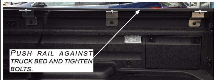
**STEP 6:** Tighten all fasteners. Repeat steps 1-5 on driver's side.
