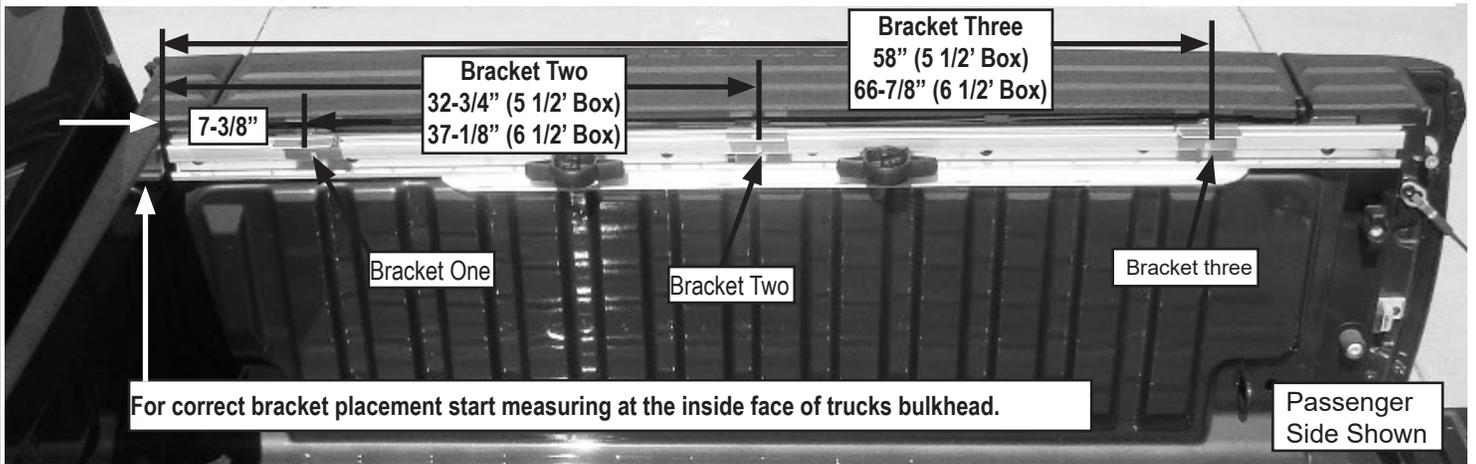
**STEP 6.** Fasten the X15 rail to the brackets with the hardware shown.
