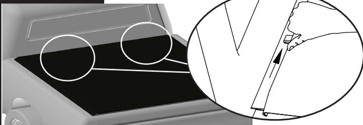
Front of cover can be opened from either the driver or passenger side of truck
