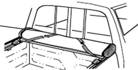
Lightbulb icon: For best results leave unrolled portion attached to the hook and loop fasteners while rolling.
