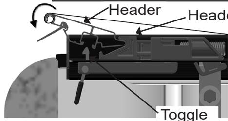
Cover closed and toggle locked in header.
