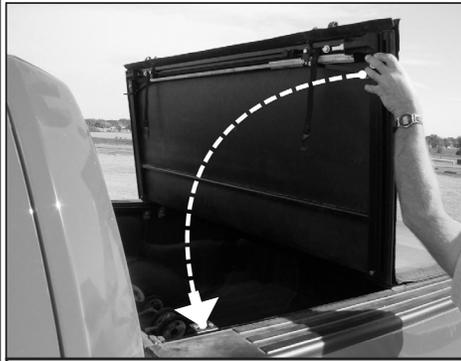
**!** Always lift upward on cover front after closing to make sure cover is securely latched.
