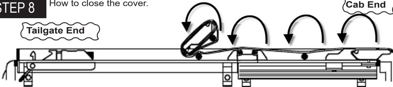
Unroll cover toward the tailgate. Rotate rear header into the header stops and press down to lock toggle into header.
