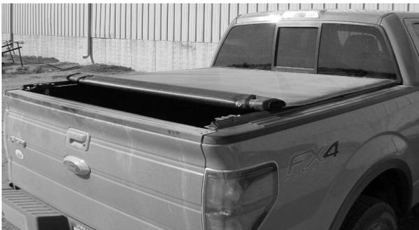
**!** **Caution**, never drive vehicle with cover unlatched at the rear or partially rolled to the front.
