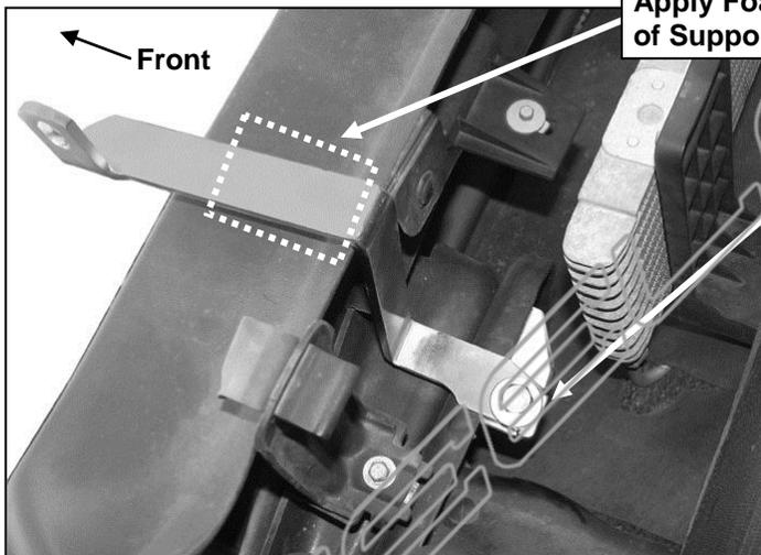
Apply Foam Tape to top and/or bottom of Support Bracket as necessary
