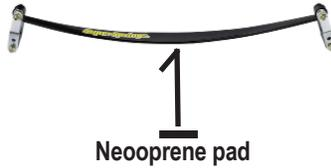
Position the neoprene pads with the adhesive side down to the bottom of the SuperSprings blades.
