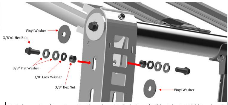
For the lower section of Upper Connecting Tube, each upright will take 2 qty. 3/8x1" hex bolts, 4 qty 3/8" flat washers, 2 lock washers, 2 hex nuts. Leave finger tight and repeat process for the remaining three corners. Install the hex bolt from the outside of the upright with one flat washer. On the inside of the upright, you'll need to install the 1 ½" vinyl spacers in between, then install one 3/8 flat washer, one 3/8 lock washer and one 3/8 hex nut. Repeat process for each upper corner.
