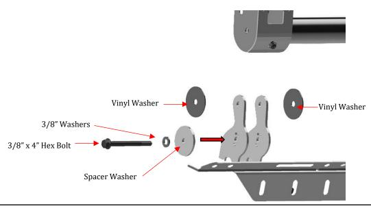
Install 3/8" x4" hex head bolt with 3/8" lock washer, 3/8 flat washer, Spacer Plate through the bottom hole of the upright. Before the bolt runs through, you will need to add (2) 2 ½' Vinyl Washer in between (one per side) \*\*\*INSTALLATION TIP\*\*\* Use painters tape to hold the vinyl washer in place when assembling it.
