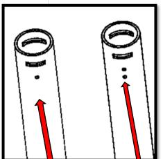
Connect Upper Multi-Core Cross bars (long) to the top connecting tube (single weep hole) using ¼ X ¾"-20 SEMS Button Head Bolts. Connect Side Multi-Core Cross bars (short) to the top connecting tube (single weep hole) using ¼ X ¾"-20 SEMS Button Head Bolts. Connect Side Multi-Core Cross bars (short) to the bottom connecting tube (two weep hole) using ¼ X ¾"-20 SEMS Button Head Bolts. Repeat process for both sides.
