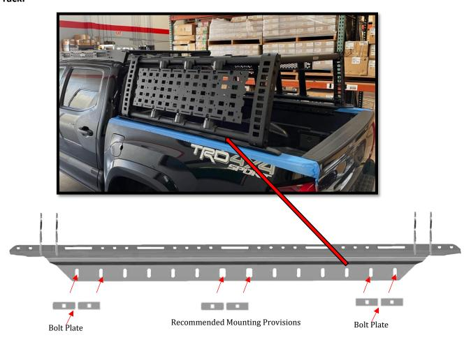
The feet on the XRS rack have a series of holes to allow for mounting in different locations. It is recommended to install the plates on the outer sides of the feet as well as in the center. This will help distribute clamping force.
