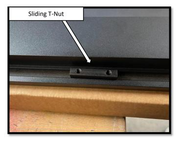
**Step 7**: Install the PASSENGER side running board. With assistance, begin by positioning the board on the front and rear motor assembly bases. Align the sliding T-Nut on the running board with the slots on the front and rear motor base. Once the T-Nuts are aligned, rotate the running board so that the T-Nuts set in the slots on the base of the arms. Repeat 1-6 to install the motor linkage assemblies and running board on the DRIVER side side.
