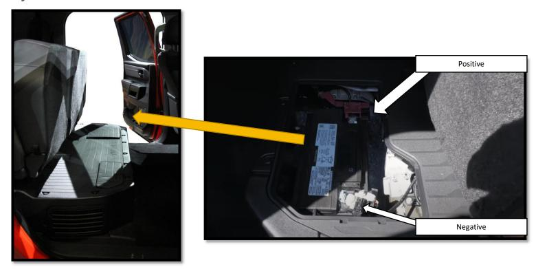
**Step 24:** Remove the 20 Amp fuses from the main positive and negative 12V power leads on the main harness. Route the power wires to the rear driver side seat. Remove battery over to expose the vehicle battery Connect the ring terminals to the battery positive and negative terminals. Install the 20 Amp fuses back into the main negative and positive power lead fuse holders. Connect the battery terminals. Begin with the positive terminal followed by the negative terminal.
