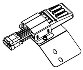
**Notice:** As shown in the picture, there is a four conductor plug, a six-conductor plug, a black two conductor plug, and a red two-conductor plug.
