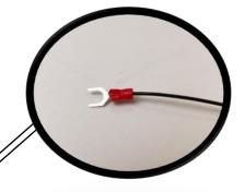
**Step 16:** The door trigger sensor harness will need a ground connection to the vehicle. Locate the seat belt assembly at the driver side b-pillar and install the ground wire under the top bolt of the seat belt assembly.
