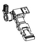
**Step 5**: Install the rear passenger side motor using (2) M8X30mm Flange Bolts, to fasten the motor to the vehicle. The hardware should be hand tightened only until snug. This will allow the motor assembly to move and align easier when installing the running board.
