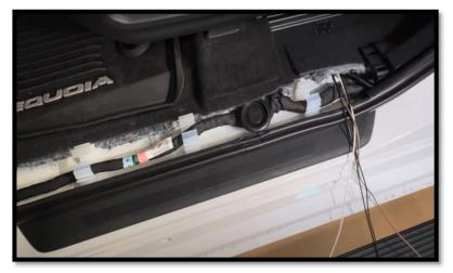
**Step 13:** On the Driver side, remove the front kick panel, front door sill trim panel and b-pillar trim panel. Go under the Driver seat and locate the rubber plug in the carpet. Pull the rear half of the carpet back to expose the oval rubber drain plug. Pull the drain plug and drill a 7/16" hole.
