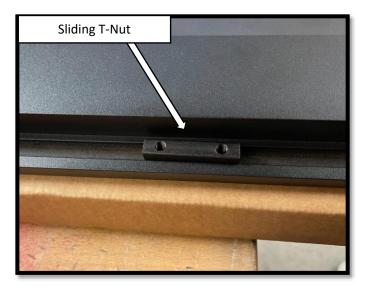
**Step 6**: Install the DRIVER side running board. With assistance, begin by positioning the board on the front and rear motor assembly bases. Align the sliding T-Nut on the running board with the slots on the front and rear motor base. Once the T-Nuts are aligned, rotate the running board so that the T-Nuts set in the slots on the base of the arms. Repeat 1-6 to install the motor linkage assemblies and running board on the DRIVER side side.
