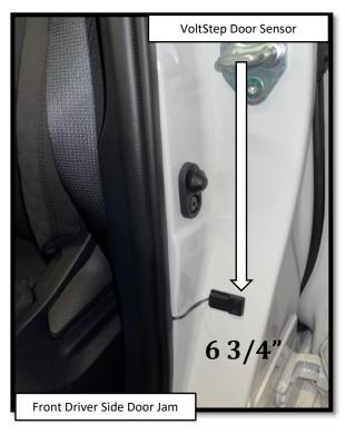
Step 17: FRONT DOOR Apply a vertically oriented strip of masking tape on the front Driver side door using the deepest part of the latch as a reference point. Make a mark 6 3/4" below the center line of the latch. Prepare the surface by cleaning with a 50/50 mix of isopropyl alcohol and water or equivalent. Once the surface is completely dry, peel the backing from the double-sided tape and stick the magnet to the door. Align the top of the magnet with the 6 3/4" mark as shown.
