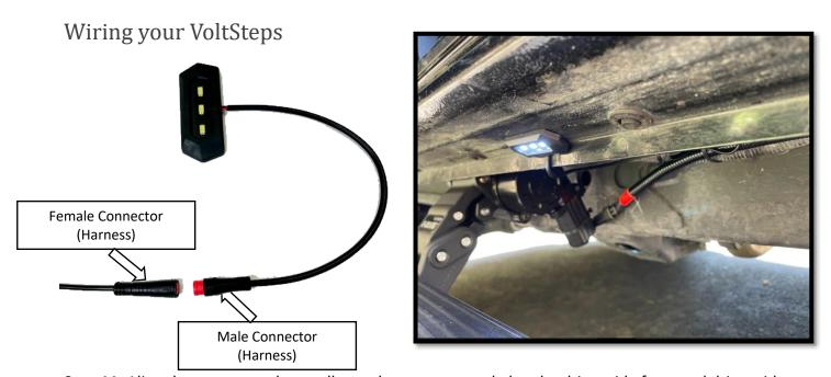
**Step 11**: Align the arrows on the small round connectors and plug the driver side front and driver side rear LED lights. Prepare the surface by cleaning with a 50/50 mix of isopropyl alcohol and water or equivalent. Once the surface is completely dry, peel the backing from the double-sided tape and stick the LEDs to the bottom side of the rocker panel. Position the LED lights at the center of the front and rear doors
