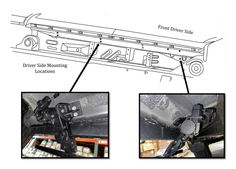
**Step 3**: Install the Rear driver side motor using (2) M8X30mm Flange Bolts, to fasten the motor to the vehicle. Use the rear center mounting hole location. The hardware should be hand tightened only until snug. This will allow the motor assembly to move and align easier when installing the running board.
