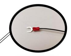
**Step 17:** The door trigger sensor harness will need a ground connection to the vehicle. Locate the seat belt assembly at the driver side b-pillar and install the ground wire under the top bolt of the seat belt assembly.
