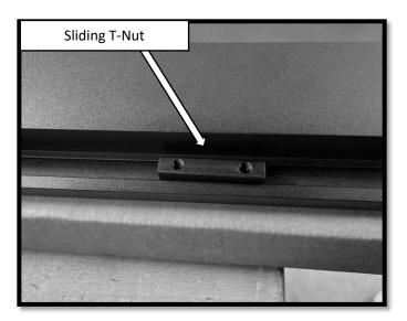
**Step 7**: Install the DRIVER side running board. With assistance, begin by positioning the board on the front and rear motor assembly bases. Align the sliding T-Nut on the running board with the slots on the front and rear motor base. Once the T-Nuts are aligned, rotate the running board so that the T-Nuts set in the slots on the base of the arms. Repeat 1-14 to install the motor linkage assemblies and running board on the PASSENGER side side.
