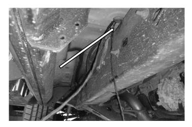
**Step 15:** Go under the vehicle and feed the door trigger signal wires (white and brown) and the disable switch wires (two black wires) into the cab. Feed the wires thru the hole in the rubber drain plug. Pop the drain plug back into the slot. Seal around the wires using RTV silicone adhesive to prevent water intrusion. These cables will run underneath the driver side seat.
