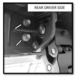
**Step 5**: Install the REAR DRIVER side motor in the last group of threaded holes. Place onto the motor base a rear driver side bracket aligning the slots. Install the assembly using (2) M8x45mm Hex Bolts, with flat and lock washers to fasten the bracket and the motor to the vehicle. The hardware should be hand tightened only until snug. This will allow the motor assembly to move and align easier when installing the running board.
