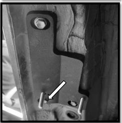
**Step 4**: Install the FRONT DRIVER side motor using (2) M8 flat washers, (2) M8 lock washers and (2) M8 hex nuts, to fasten the motor to the bracket. The hardware should be hand tightened only until snug. This will allow the motor assembly to move and align easier when installing the running board.
