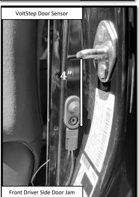
Step 18: FRONT DOOR Apply a vertically oriented strip of masking tape on the front Driver side door using the deepest part of the latch as a reference point. Make a mark 3.5" below the center line of the latch. Prepare the surface by cleaning with a 50/50 mix of isopropyl alcohol and water or equivalent. Once the surface is completely dry, peel the backing from the double-sided tape and stick the magnet to the door. Align the top of the magnet with the 4" mark as shown.
