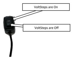
**Step 25:** Open the Driver side door and keep the door open. Flip the disable switch to the Off position. This will signal the running boards to retract to the stowed position and it will disable any further operation until the switch is flipped to the On position.
