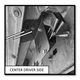
**Step 6**: Install the CONTROL MODULE on driver side center mount side motor using (2) M8X25mm Flange Bolts.
