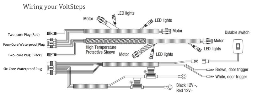
**Step 10:** Route the electrical harness from the controller along the frame rail of the vehicle. Connect the male plug connector on the wire harness into the female socket on the motors. The harness is labeled to show where to plug each male connector to the female connector. For example, Front Left is for the front Driver side motor and Rear Left for the rear Driver side motor. Use supplied zip-ties to secure harness to the frame rail.
