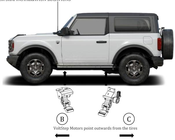
**Step 8**: Repeat Steps 1-4 to install the motor linkage assemblies on the passenger side. Repeat steps 6-7 to install running board on the driver side.
