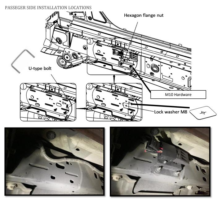
**Step 5**: Locate the hole near the center of the cab on the Passenger side frame of the vehicle. Insert the bolt plate into the elongated hole and secure it using the M8 plastic washer. Position the control module against the bolt plate and secure using (2) M8 nuts, flat washer and lock washer.
