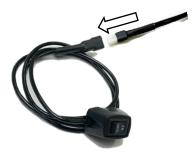
**Step 21:** Locate the black wires for the disable switch and feed them to your desired mount location. Prepare the surface by cleaning with a 50/50 mix of isopropyl alcohol and water or equivalent. Once the surface is dry, peel the backing from the double-sided tape and stick the disable switch on the lower dash panel. Plug the disable switch connector into the black wire harness and tuck the extra wire behind the lower dash panel.
