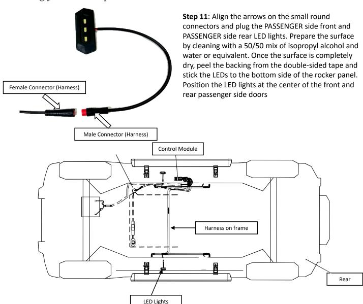
**Step 12**: Route the motor and LED wire harness from the controller to the Driver side frame rail of the vehicle. When routing the harness keep clear from any moving parts and avoid direct contact with the exhaust system.
