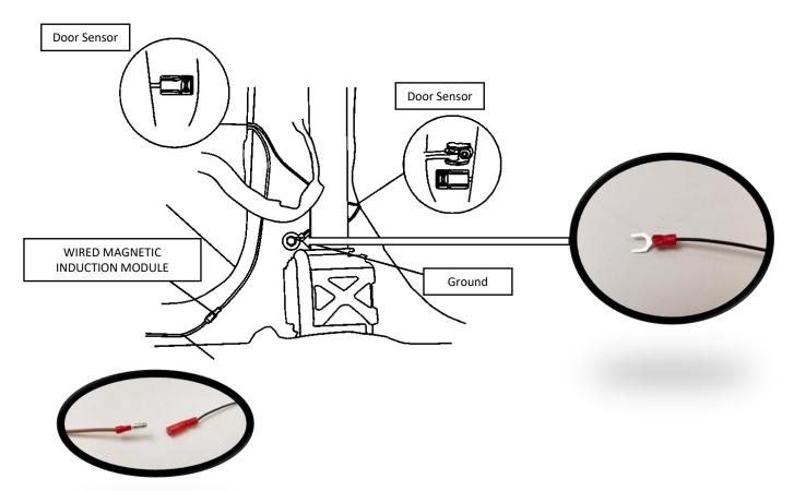
**Step 14:** The door trigger sensor harness will need a ground connection to the vehicle. Locate the seat belt assembly at the driver side b-pillar and install the ground wire under the top bolt of the seat belt assembly. Connect the snap-in bullet connector to the brown wire on the Passenger side b-pillar.
