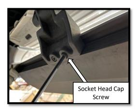
**Step 7**: Determine where you want to position the board and secure the running board to the arms using the (2 per bracket) M6x25 socket head cap screws. Using a torque wrench, tighten to 9 ft-lbs. Step # With the running board is installed, fasten the hardware on the Driver side front and rear motor assemblies. Using a torque wrench, tighten the mounting hardware to 18 ft-lbs.
