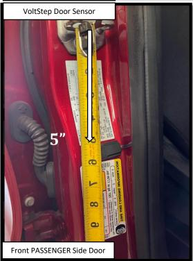
**Step 16: FRONT DOOR** Apply a vertically oriented strip of masking tape on the front PASSENGER side door using the deepest part of the latch as a reference point. Make a mark 5" below the center line of the latch. Prepare the surface by cleaning with a 50/50 mix of isopropyl alcohol and water or equivalent. Once the surface is completely dry, peel the backing from the double-sided tape and stick the magnet to the door. Align the top of the magnet with the 5" mark as shown.
