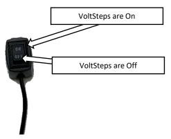
**Step 23:** Open the PASSENGER side door and keep the door open. Flip the disable switch to the Off position. This will signal the running boards to retract to the stowed position and it will disable any further operation until the switch is flipped to the On position.
