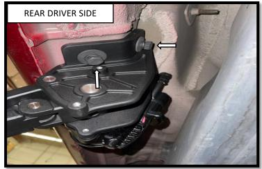
**Step 5**: Install the rear driver side motor using (2) M10x30MM hex bolts M10 Lock Washer, M10 Flat Washer, to fasten the motor to the truck. The hardware should be hand tightened only until snug. This will allow the motor assembly to move and align easier when installing the running board.
