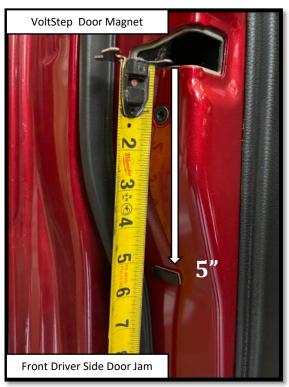
Step 17: FRONT DOOR Apply a vertically oriented strip of masking tape on the front driver side door using the deepest part of the latch as a reference point. Make a mark 5" below the center line of the latch. Prepare the surface by cleaning with a 50/50 mix of isopropyl alcohol and water or equivalent. Once the surface is completely dry, peel the backing from the double-sided tape and stick the magnet to the door. Align the top of the magnet with the 5" mark as shown.
