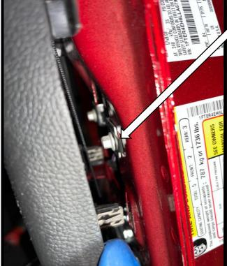
**Step 16:** The door trigger sensor harness will need a ground connection to the vehicle. Locate the seat belt assembly at the driver side b-pillar and install the ground wire under the top bolt of the seat belt assembly.
