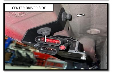
**Step 7**: Locate the threaded holes near the center of the cab on the Driver side of the truck. Install the controller bracket using (2) M10x25MM hex bolts M10 Lock Washer, M10 Flat Washer, to fasten the control module to the truck.
