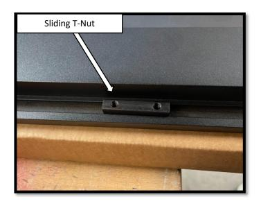
**Step 8**: Install the driver side running board. With assistance, begin by positioning the board on the front and rear motor assembly bases. Align the sliding T-Nut on the running board with the slots on the front and rear motor base. Once the T-Nuts are aligned, rotate the running board so that the T-Nuts set in the slots on the base of the arms. Repeat Steps 3-6 to install the motor linkage assemblies and running board on the Driver side.
