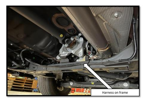
**Step 13**: Route the motor and LED wire harness from the controller to the Passenger side frame rail of the vehicle. When routing the harness keep clear from any moving parts and avoid direct contact with the exhaust system.
