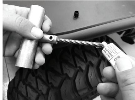
**3** Insert Reamer in puncture. Cycle the reamer through the puncture wound while twisting the reamer. This will open the rubber slightly while repositioning the steel belts to make room for the plug.
