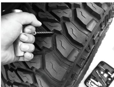
**4** Thread a plug through the T-Handle Insertion Needle. Adjust needle to middle of the plug. Flattening the end of the plug will help get it started through the needle.
