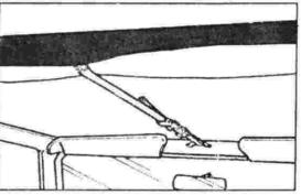
STEP FOUR: ADD THE FEMALE SIDE OF THE QUICK RELEASE BUCKLE (SUPPLIED WITH BRIEF) TO THE CENTER STRAP IN THE MIDDLE OF THE WINDSHIELD FRAME. PULL THE CENTER STRAP FORWARD AND THREAD THROUGH THE MALE SIDE OF THE QUICK RELEASE. TIGHTEN THE CENTER STRAP.
