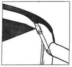
STEP THREE: LAY THE BACK OF THE BRIEF OVER THE MAIN BAR OF THE ROLL BAR AND PULL THE REAR CORNER STRAPS UNDER THE REAR ROLL BAR BRACE AND UP TO THE QUICK RELEASE BUCKLE. THREAD THE STRAP THROUGH THE QUICK RELEASE BUCKLE. DO NOT TIGHTEN COMPLETE. REPEAT THE ABOVE INSTRUCTION ON THE OPPOSITE SIDE. NOW TIGHTEN BOTH SIDES COMPLETELY.
