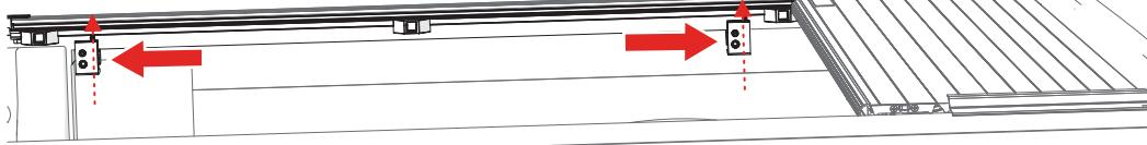
**3c** - Once the clamps (G) are correctly positioned, rubber shims need to be placed between the steel flange of the truck bed and the plastic flange of the truck bed rail cap. The shims need to be placed directly behind the clamps.
