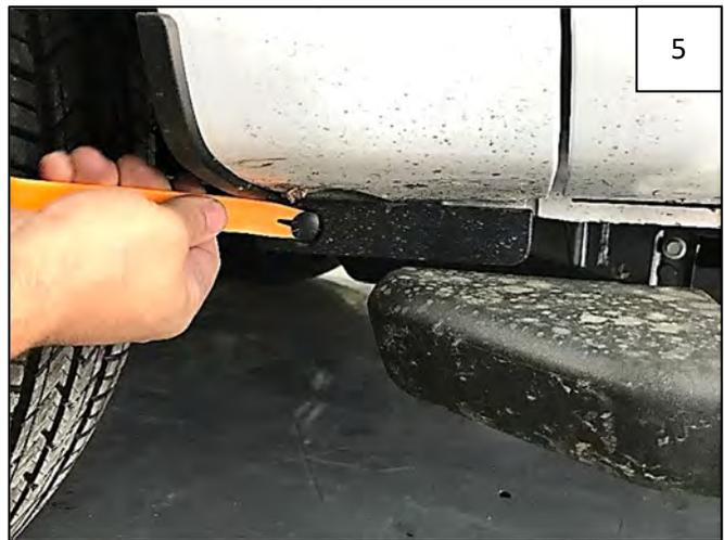
Use a Pry Tool to disengage factory push pin on underside of plastic trim as shown.
