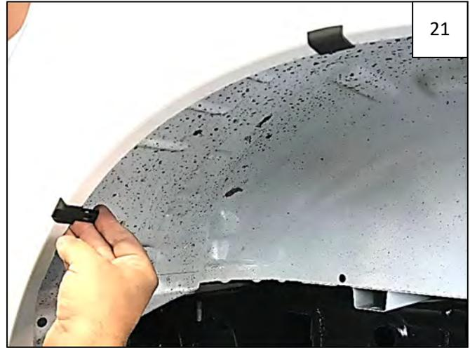
Slide a supplied Long "U" Clip over each foam tab. Clip will overhang wheel well lip on both inner and outer surface. Clip hole should be centered approximately over mark made in Step 18.
