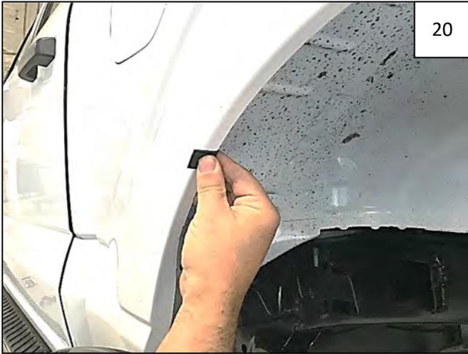
Peel backing from supplied Foam Tab. Center a Foam Tab over each mark made in Step 18, folding each tab over the wheel well lip. Press to adhere.
