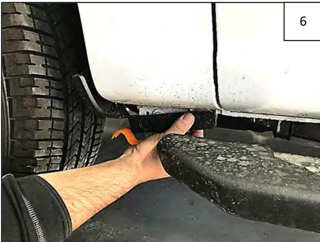
Remove and discard plastic trim by pulling firmly away from vehicle, disengaging a factory clip inside.
