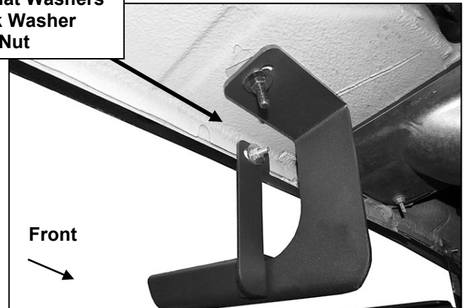
(Fig 12) Mark and drill hole through pinch weld. Attach top of Driver/left rear Support Bracket to back of pinch weld. Reinstall Running Board
