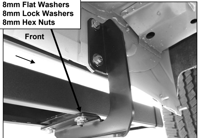
(Fig 8) Driver/left front mounting Bracket installed
