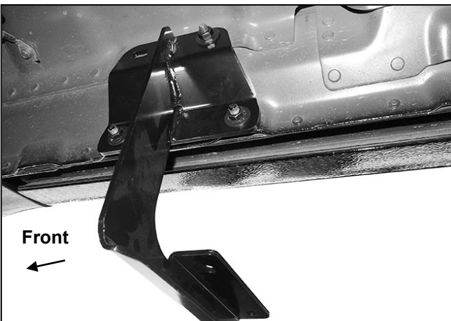
(Fig 5) Passenger/right front Bracket installed
