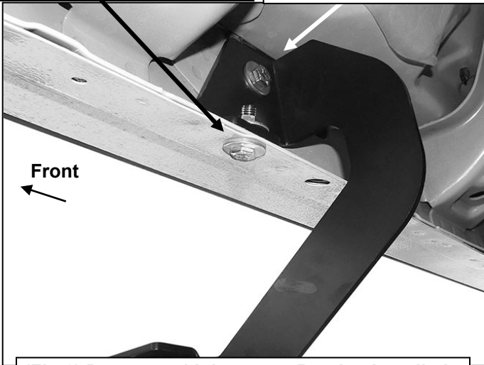
(Fig 6) Passenger/right center Bracket installed
