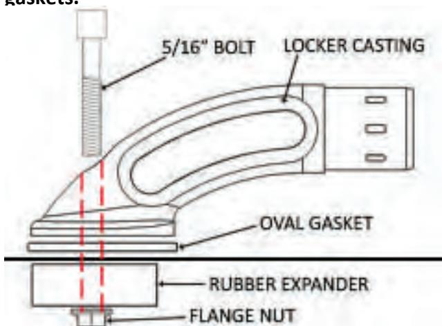
Install the Allen head bolt through the hole in the Standard Locker casting, plastic oval gasket, and rubber expander. Screw the threaded back plate onto the bolt and snugly tighten the plate against the rubber expander.
