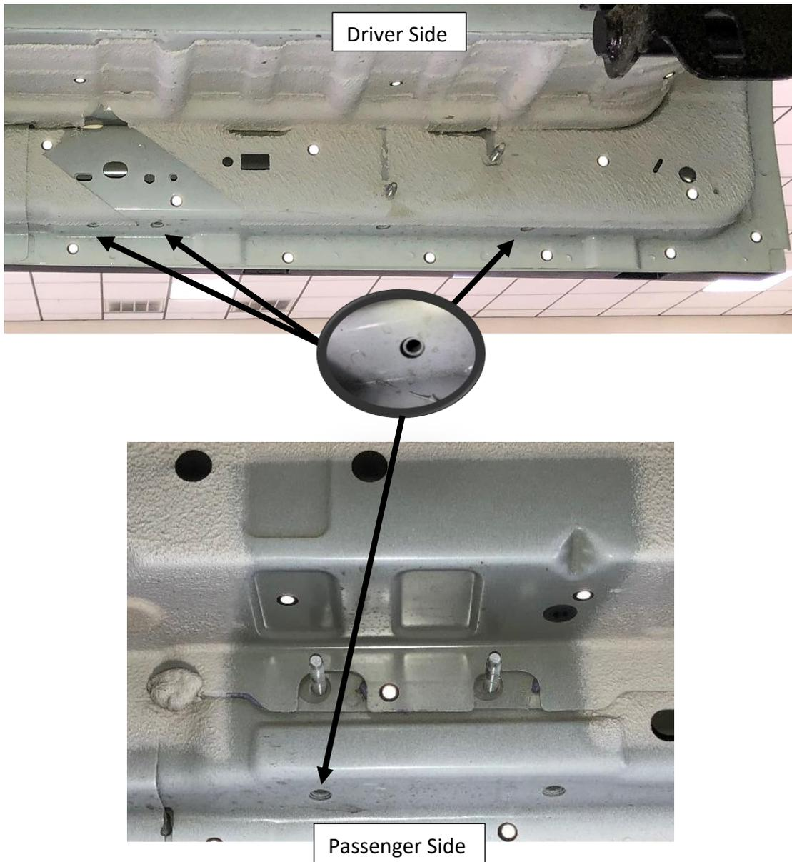
**Step 3:** Each M8 hole location identified in step 2 will be threaded using the supplied M8x20mm hex head thread cutting bolts. To do this you will need a powered nut driver, 13mm short socket and Ratchet wrench.
