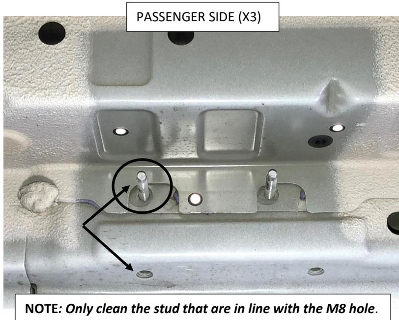
**Step 2:** There are six factory M8 mounting holes that will need to be threaded. Three on the **driver side** and three on the passenger side. The three on the **passenger side** will be located directly under the M8 studs that were cleaned in the step 1.
