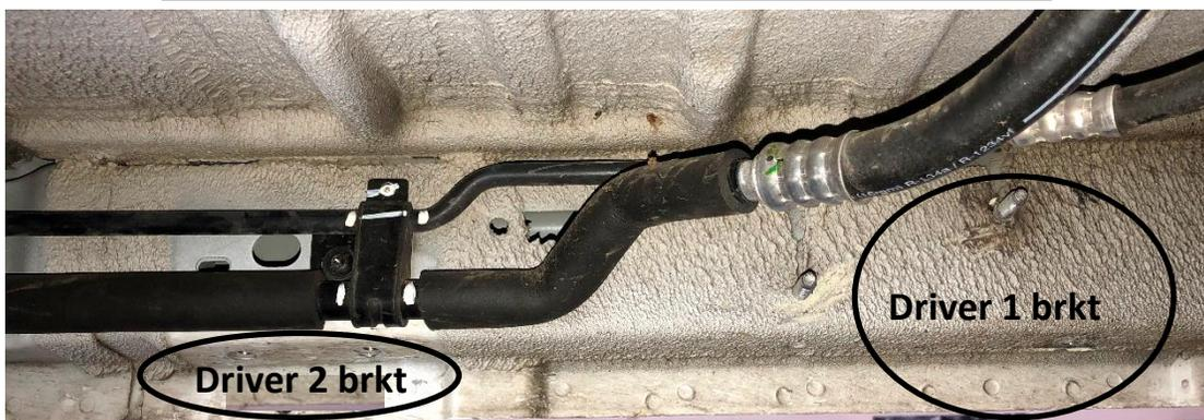
**Step 1:** Install **Driver #1 brkt** on the factory-threaded stud and loosely fasten with one of the supplied M8 flanged nuts. Next, install one of the M8x20mm hex bolts, lock washer and flat washer to the lower mount and loosely tighten.
