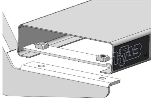
**Step 10:** After final adjustment, tighten all running board threaded mounts.
