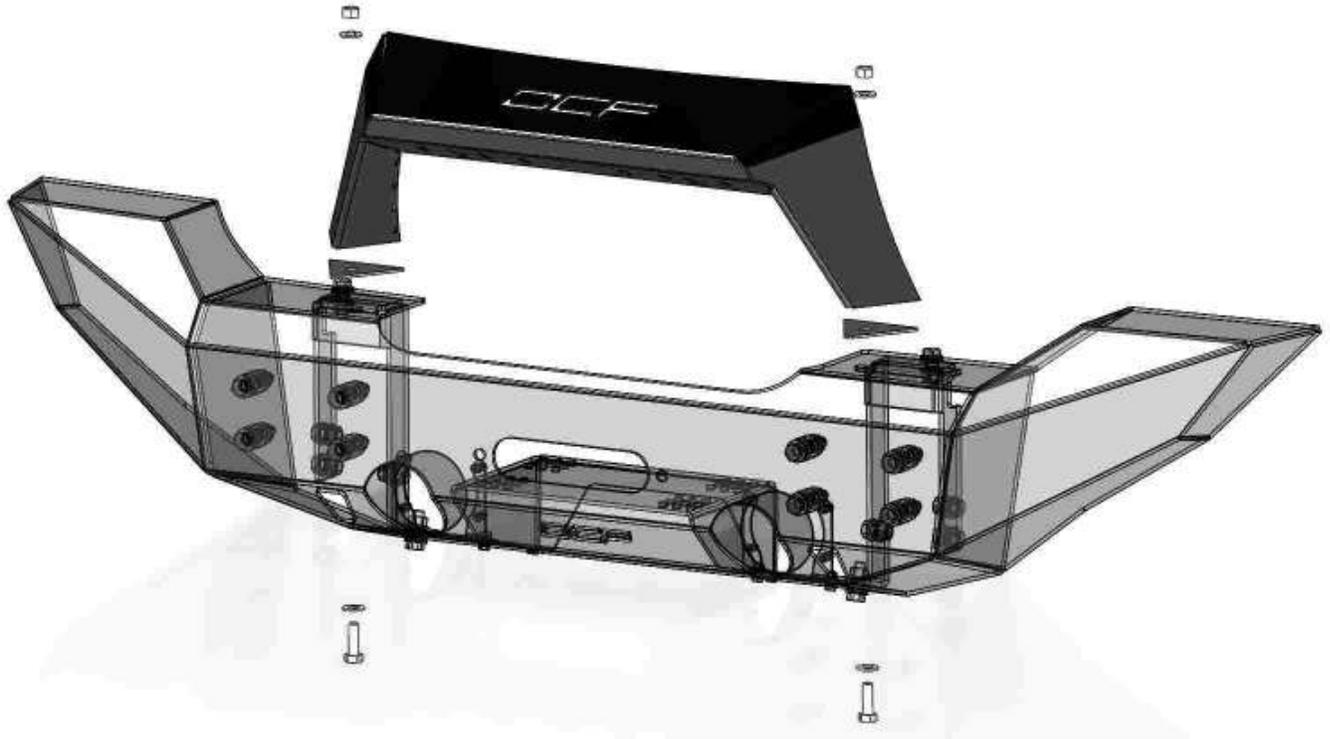
1. Loosely Place the two **Gaskets** between the **Light Bar** and the top face of the bumper.
