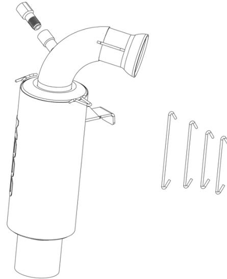
NOTE: To avoid exhaust leaks use a high heat silicone to seal all connections between the expansion chambers and the muffler. Monitor the exhaust for leaks during the first 200 miles after your installation and re-apply silicone where necessary. We suggest having your local snowmobile mechanic or performance shop install this product.
