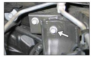
18. Remove the front fender mounting bolt shown. **NOTE: This bolt will used in a later step.**
