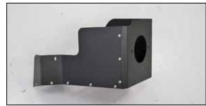
11. Choose the appropriate heat shield wall for year model of the vehicle and attach to the heat shield as shown using the provided hardware.
