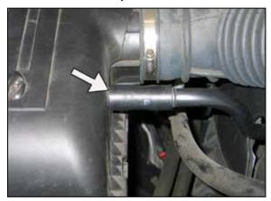
4. Disconnect the crank case vent hose from the air
