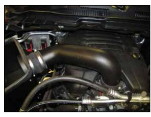
25. Install the K&N® intake tube into the silicone hump hose and then into the silicone hose at the throttle body. Align the heat shield assembly for proper fit and then tighten the heat shield mounting bolts. Also secure the hose clamps securing the intake tube.
