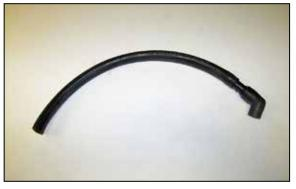
8. Remove the factory 45 deg. elbow from the factory CCV hose assembly. Assemble the K&N $^{\odot}$  CCV hose, Union and factory 45 deg. elbow as shown.
