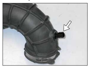
23. Remove the inlet air temperature sensor from the stock intake tube.
