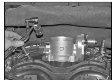
9. Disconnect the TPS sensor electrical connection from the throttle body.
