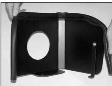
16. Install the edge trim onto the heatshield as shown.
