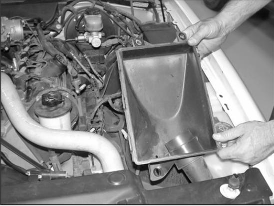
9. Remove air box bottom from vehicle as shown. **NOTE: K&N Engineering, Inc., recommends that customers do not discard factory air intake.**
