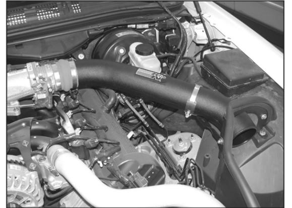
20. Install the K&N® intake onto the throttle body, then secure the tube to the saddle bracket assembly with the provided hose clamp. **NOTE: Do not tighten completely.**
