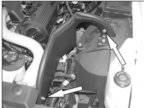
15. Install the heat shield onto the vehicle and attach to the outer brackets as shown.
