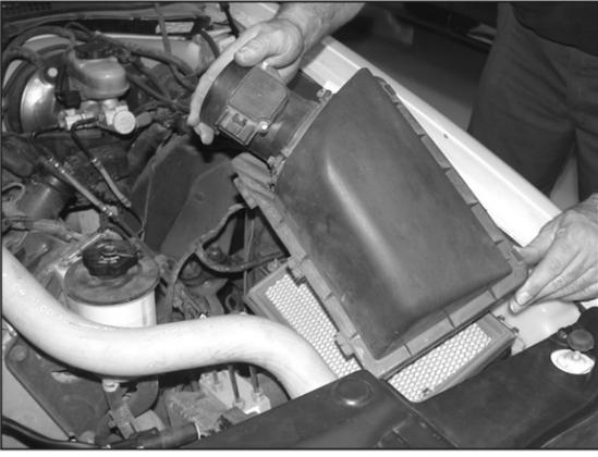
7. Release the 2 clips which retain the air box lid, then remove the lid and filter from the vehicle.
