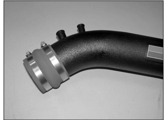
19. Install the provided silicone hump hose (087121) onto the K&N® intake tube with the provided hose clamps.
