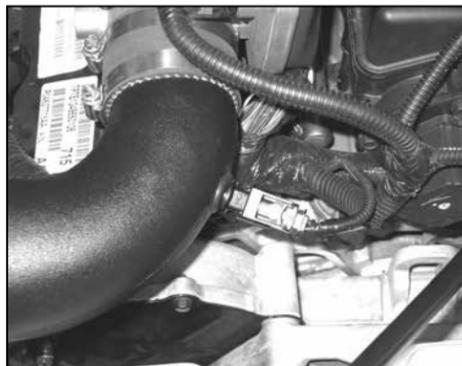
17. Re-connect the air temperature sensor electrical connection.
