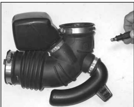
13. Remove the air temperature sensor from the stock intake tube as shown.
