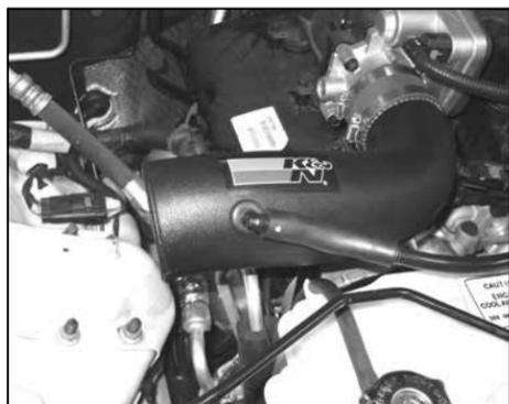
18. Connect the crank case vent hose to the 90° fitting installed into the K&N® intake tube as shown.
