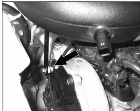
16. Secure the tube mounting bracket to the timing cover with the provided hardware as shown.
