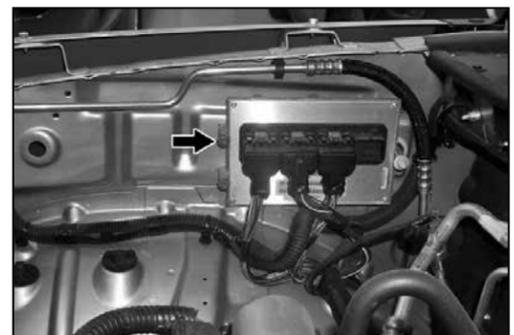
7a. On 2008 and later model vehicles, remove the ECU mounting bolt shown.
