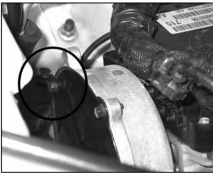
8. Remove the timing cover bolt (shown).
