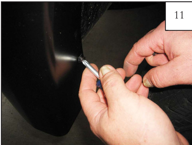
Install four supplied Screws (SW1-0050) through remaining holes and into clips installed in Step 9, working from front to back of wheel well.
