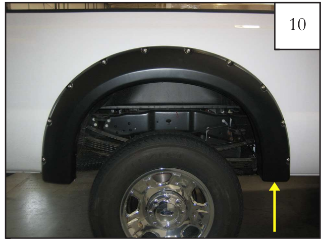
Place flare on fender and reinstall bolt removed in Step 5.
