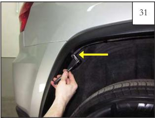
Using a 10mm socket and ratchet or a 10mm wrench, remove factory screw at indicated location in image above. Retain screw for reinstallation.
