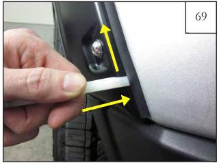
Using flat end of supplied Edge Trim Tool (ET1-0002), seat edge trim against vehicle by inserting straight end between edge trim and flare at one end. Slide the tool along entire length of edge trim while pressing in towards the vehicle surface.
