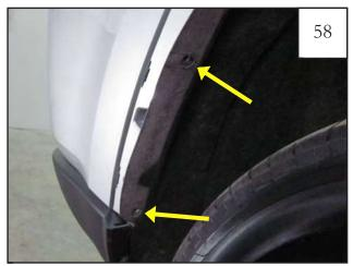
At rear of wheel well, pull back factory liner and install (2) Clips (CL1-0022) over holes in plastic bumper at locations indicated in image above (Black Plastic Tabs are not needed on these plastic bumper hole locations). Replace factory wheel well liner back to original position.
