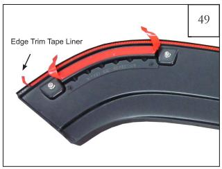
Remove 1-2 inches of red tape liner from each end of installed edge trim and fold towards outside of the Door Flare. NOTE: ONLY REMOVE 1-2" OF TAPE LINER FROM THE <u>EDGE TRIM</u>. DO NOT REMOVE LINER FROM TAPE PADS. SEE NEXT STEP.
