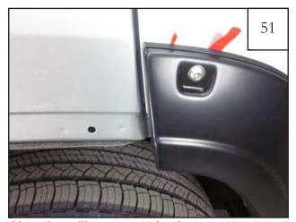
Place Door Flare on vehicle aligning with edge of door seam and installed Inner Door Piece. *Note:* Ensure all tape liners are visible.
