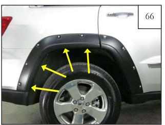
Screw/Clip locations (4 places). Ensure flare is properly aligned on vehicle. Style lines of Rear Door Flare and Rear Main Flare should match. Once properly aligned tighten all fasteners.
