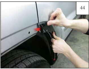
Hold Inner Door Piece against vehicle aligning upper hole with factory hole in sheet metal and the remaining three holes with grommets installed in step 41. Install (1) provided Push Retainer (RV1-0014) into top hole to secure Inner Door Piece to vehicle. *Note: Be sure to*
