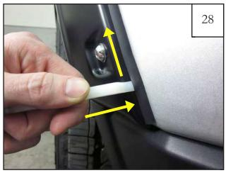
Using flat end of supplied Edge Trim Tool (ET1-0002), seat edge trim against vehicle by inserting straight end between edge trim and flare at one end. Slide the tool along entire length of edge trim while pressing in towards the vehicle surface.
