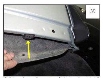
Pull down factory liner at top of wheel well and install (2) Black Plastic Tabs (MT1-0014) and 2 Clips (CL1-0022) over factory holes (2 places). The hole in the Clip should align with the factory hole in the sheet metal covered by the Plastic Black Tab.
