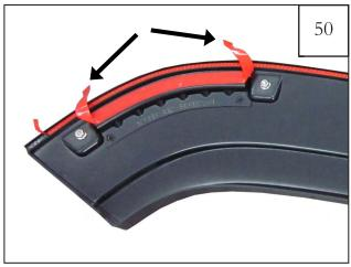
Fold tape leaders of tape pads towards the outer edge of Door Flare. **DO NOT REMOVE TAPE LINER FROM TAPE PADS AT THIS TIME.**
