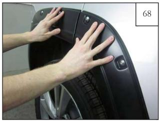
After the red liner is removed, *firmly* press the Door Flare and Rear Main Flare toward the vehicle for 10 seconds to adhere the tape to the vehicle surface. Repeat this process for entire length of Flares. The vehicle surface temperature must be between 65-110° F for proper adhesion. Allow 24 hours for full adhesion.
