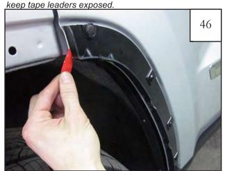
Remove red tape liner from Inner Door Piece.
