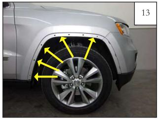
Use a pry tool to remove factory fasteners at locations indicated in image above. A supplied Black Plastic Tab (MT1-0014) and Clip (CL1-0022) will be installed at these locations.
