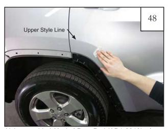
Using provided Alcohol Prep Pad (AD1-0010), clean sheet metal for Rear Door Flare installation. Use upper style line on door as a guide.
