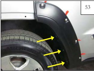
Ensuring part is aligned properly, start (3) Screws (SW1-0056) through Door Flare and into Clips on installed Inner Door Piece at indicated locations. Do not fully tighten at this time.
