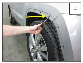
Use a pry tool to remove any remaining factory fasteners that may have stayed on the vehicle during the removal process. Straighten the front wheels once all fasteners have been removed.
