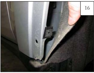
Place supplied Metal Clip (CL1-0022) over Black Tabs installed in step 15. The hole in the Clip should align with the factory hole in the sheet metal covered by the Plastic Black Tab.
