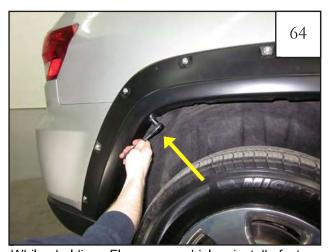
While holding Flare on vehicle, install factory fasteners removed in Step 31 & Step 57 using a 10mm socket and wrench. Do not fully tighten at this time.
