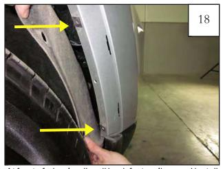
At front of wheel well, pull back factory liner and install (2) Clips (CL1-0022) over holes in plastic bumper as indicated in image above. Replace factory wheel well liner back to original position.
