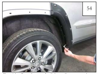
If part is aligned properly, tighen all screws using a Phillips Head Screwdriver. *Note: You can open door for better access if needed.*
