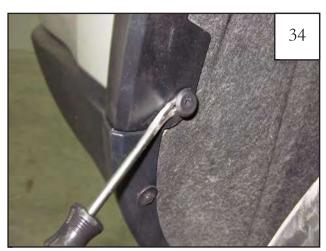
Using a utility knife and/or pry tool, remove the bottom factory fastener indicated in Step 32.
