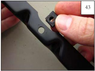
Install (4) provided Clips (CL1-0023) on Inner Door Piece at locations indicated in previous step.
