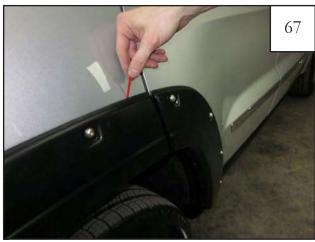
Remove the red tape liner from edge trim on the Door Flare and Rear Main Flare. *Note: Be careful not to tear red tape liner during removal process.*
