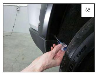
Using a Stubby or Right Angle Screwdriver, install supplied Screws (SW1-0056) thru flare and into clips installed in steps 58 & 59. Do not fully tighten at this time.
