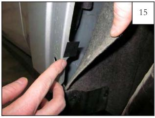
Pull adhesive liner from supplied Plastic Black Tabs (MT1-0014) and fold over the factory hole locations to cover and adhere to each side of the sheet metal (5 places refer to Step 13).
