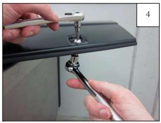
Fully tighten using an 8mm wrench or 3/8 ratchet with a 8mm socket for the Nyloc Nut, and use the supplied Torx Bit (SW1-0052) and wrench for the Bolt. Repeat for remaining pockets.
