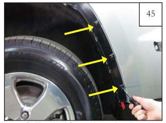
Use a Phillips Head Screwdriver to install provided Screws (SW1- 0044) into the three remaining hole locations. Do not fully tighten at this time.
