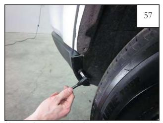
Use an 8mm socket and wrench to remove the factory screw at rear of wheel well on lower bumper.
