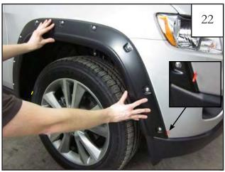
Hold the front Flare onto vehicle ensuring tape liners are exposed on both side of flare.
