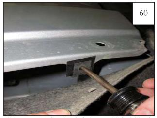
Using an awl tool make a hole thru each Black Plastic Tab (MT1-0014) using the hole in the clip as a guide. Replace factory wheel well liner to original position.
