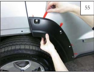
Remove 1/2" wide red tape liner from the upper and lower tape pads on the Door Flare. **NOTE: DO NOT REMOVE TAPE LINER FROM <u>EDGE TRIM</u> AT THIS TIME.**
