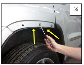
Use a pry tool to remove any remaining factory fasteners that may have stayed on the vehicle during the removal process. Remove factory fasteners from wheel well liner (2 places indicated by arrows).
