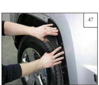
After the red liner is removed, *firmly* press the Inner Door Piece toward the vehicle for 10 seconds to adhere the tape to the vehicle surface. Repeat this process for the entire length of the part. The vehicle surface temperature must be between 65-110° F for proper adhesion. Once adhered, fully tighten all screws.
