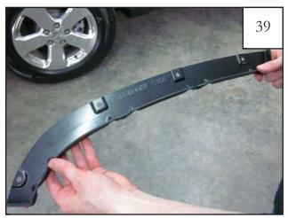
Locate the Door Flare Inner Piece. The Inner Door Pieces are marked "Passenger Side" & "Driver Side".
