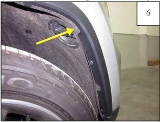
Using a 10mm socket and wrench, remove factory screw at indicated location in image above. Retain screw for reinstallation.
