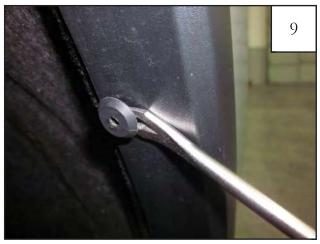
Using pry tool, remove factory fasteners drilled in previous step.
