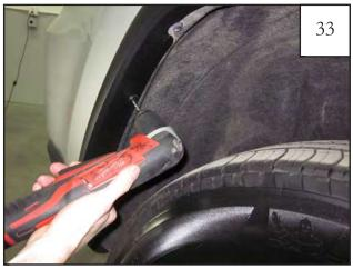
Using a 1/8" Drill bit, Drill out the center of top factory fastener in the rear of the wheel well indicated in Step 32. Use a pry tool to fully remove fastener.
