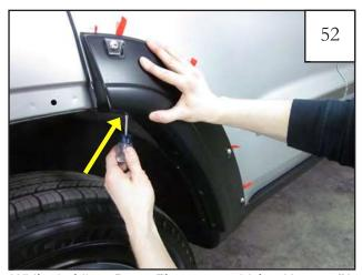
While holding Door Flare on vehicle, Use a #2 Phillips Stubby Screwdriver and install (1) provided Screw (SW1-0056) at top most location indicated in image. Do not fully tighten at this time.
