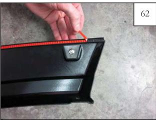
Pull back 1-2 inches of red tape liner from each end of installed edge trim and fold towards outside of the flare
