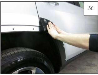
Firmly press the door flare toward the vehicle for 10 seconds to adhere the tape to the vehicle surface. The vehicle surface temperature must be between 65-110° F for proper adhesion. Allow 24 hours for full adhesion.
