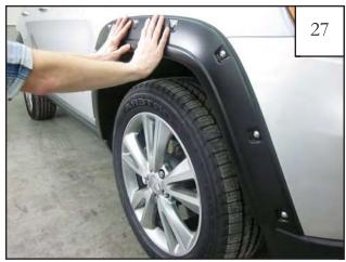
After the red liner is removed, *firmly* press the flare toward the vehicle for 10 seconds to adhere the tape to the vehicle surface. Repeat this process for the entire length of the flare. The vehicle surface temperature must be between 65-110° F for proper adhesion. Allow 24 hours for full adhesion.
