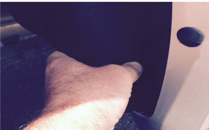
5. Insert the lower flap sections of the Wheel Well Guard into the fender well behind the fender well lip. Perform this step for both the front and rear lower flap sections.
