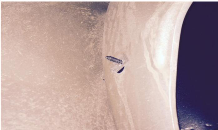
8. At locations A and D install the #10 SEM screws through the Wheel Well Guard and the slotted factory hole and into a U-clip on the backside of the sheet metal.
