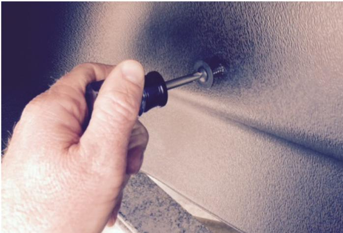
7. Align the holes in the Wheel Well Guard at locations B and C with the factory screw locations with the U-clips and install the #10 SEM screws using a phillips head screwdriver.
