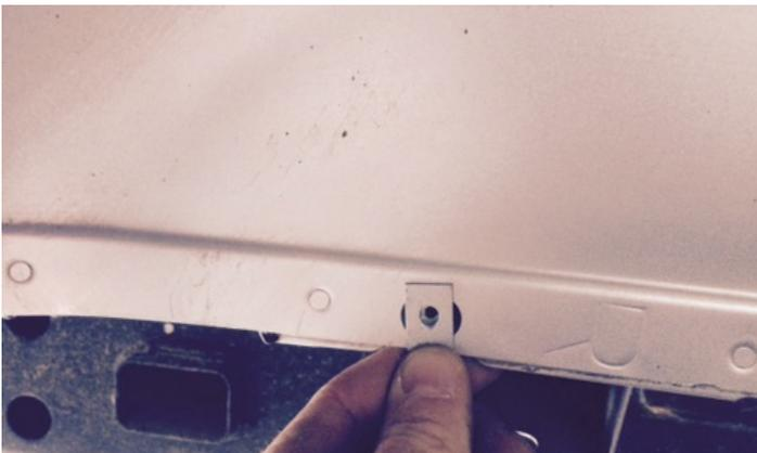
2. Install a u-clip over the factory hole at location B and C.
