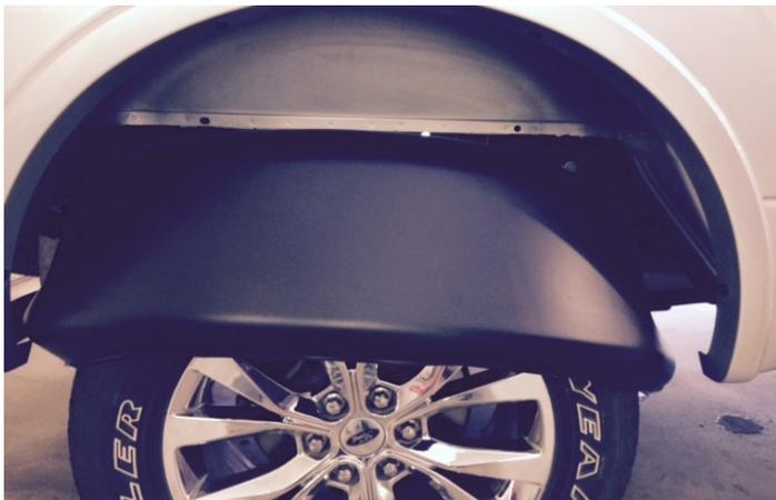
3. Insert the Wheel Well Guard into the rear wheel well opening over the tire.
