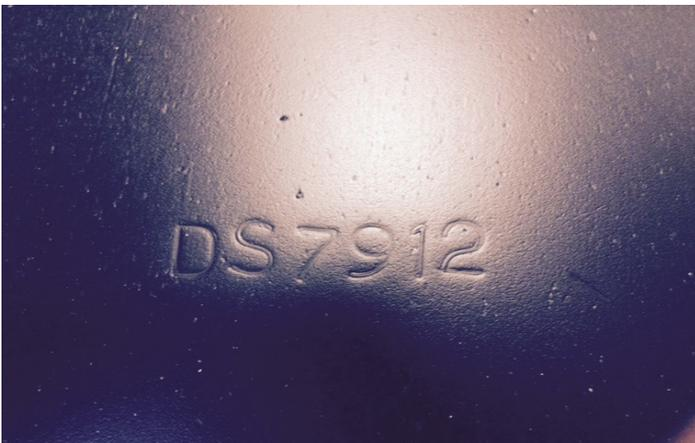
1. Check part number on the top of the Wheel Well Guard and identify DS & PS to determine which side to install.
