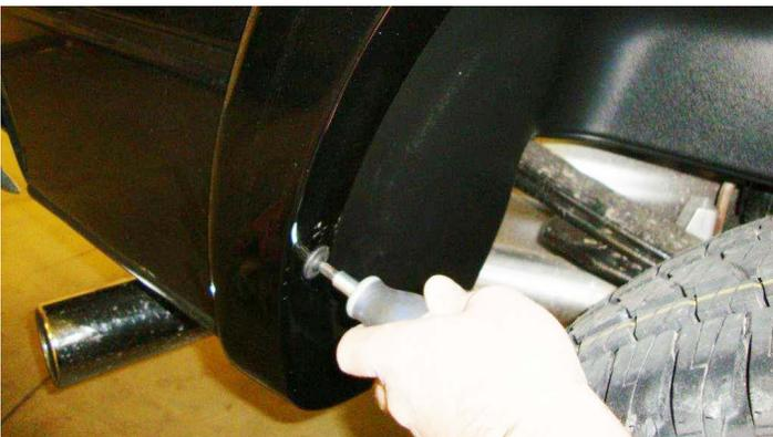
9. Installation of SEM screws and U-Clips on lower fender:
