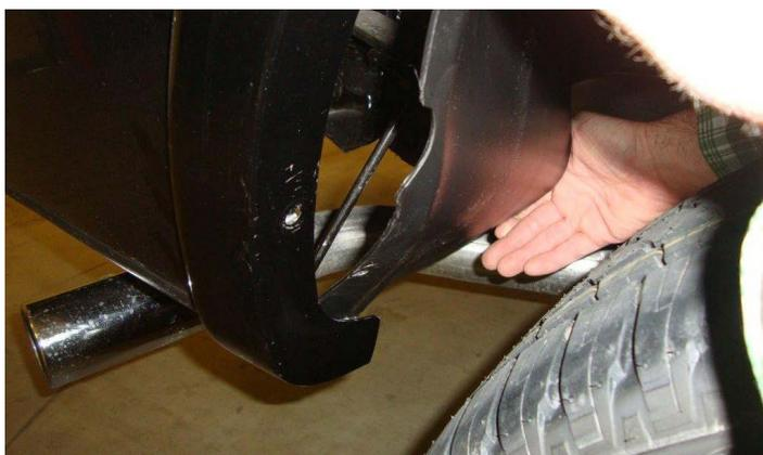
5. Insert the lower flap sections of the Wheel Well Guard into the fender well behind the fender well lip. Perform this step for both the front and rear lower flap sections.
