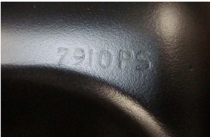
2. Verify that you're installing the correct Wheel Well Guard by checking the part no. located on the backside on the part.
