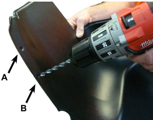
1. There are 3 installation locations marked with an indent on each 7910 Wheel Well Guard. Depending on your vehicle configuration, 1 or 2 of these locations will need to be drilled with a 1/4" Drill Bit prior to installation.
