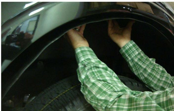
4. Push The Wheel Well Guard up into the wheel well opening.
