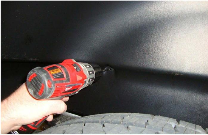
7. Push the Wheel Well Guard up until it rests against the inside of the fender well. Drill 1/8" holes at locations C and D.
