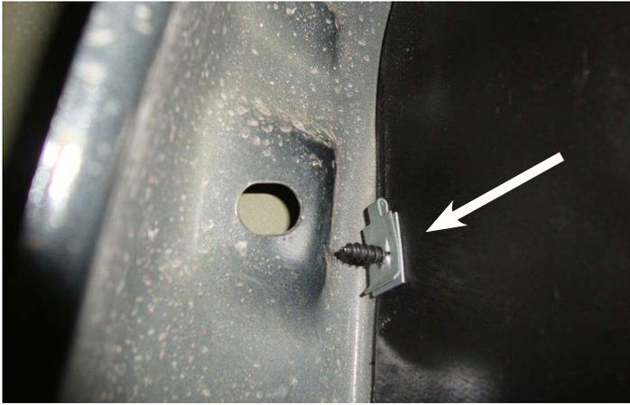
10. Do not clip the U-Clip over the Wheel Well Guard. The U-Clip functions as a “nut” and is placed on top of the Wheel Well Guard at location A OR locations B and E (depending on your vehicle configuration).
