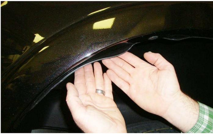
6. Tuck the remaining portion of the Wheel Well Guard behind the fender lip all the way around the fenderwell opening.
