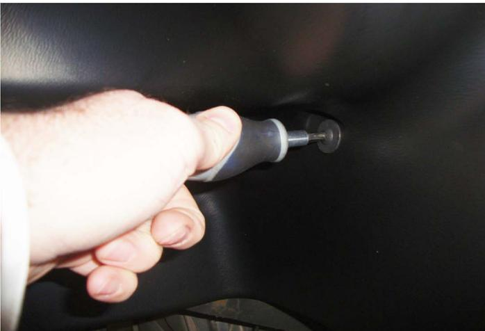
8. Install #10 SEM screws at locations C and D, through the Wheel Well Guard and into the pre-drilled sheet metal holes. Leave screws loose until all fasteners are installed.
