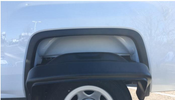
4. Insert the Wheel Well Guard into the fender opening.
