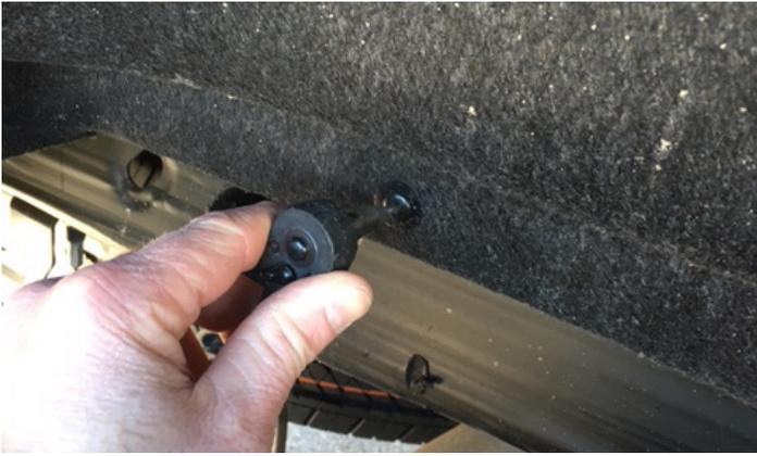
2. Remove the factory Torx head screws that hold the factory carpeted wheel well liner in place and remove the factory wheel well liner.
