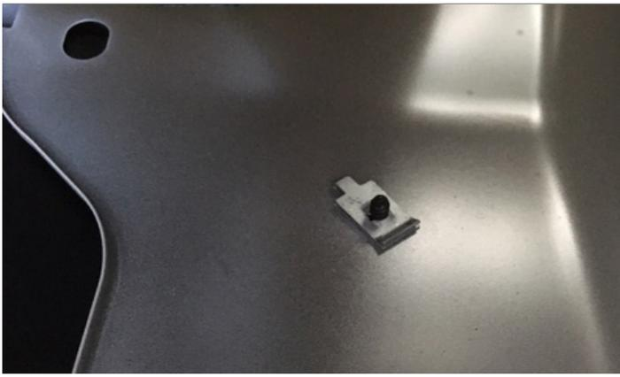
10. At locations A, B, E, and F install a SEM screw through the Wheel Well Guard and hole in the sheet metal and into the supplied u-clip on the backside on the metal.
