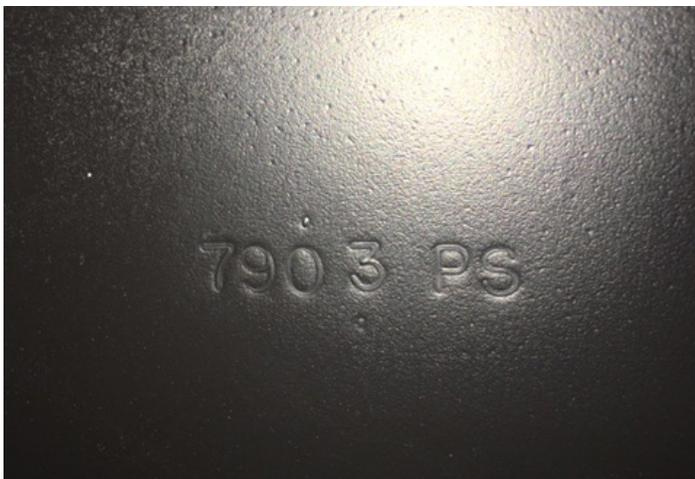
1. Check part number on the top of the Wheel Well Guard and identify DS & PS to determine which side to install.
