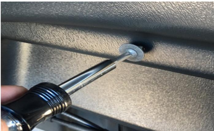
9. If your vehicle was not equipped with a factory wheel well guard, install the supplied SEM screws at locations C and D through the Wheel Well Guard and into the u-clips that are clipped over the sheet metal.
