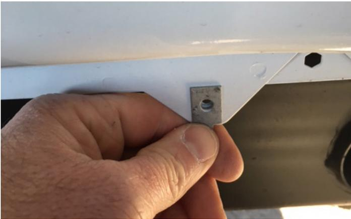
3. If your truck was not equipped with factory wheel well liners install a u-clip at locations C and D by clipping the u-clip over the tab and aligning with the factory hole.
