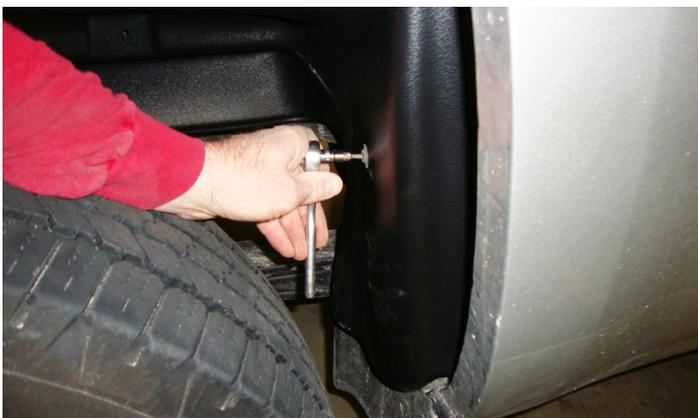
8. Align the 4 holes in the Wheel Well Guard with the factory screw locations and install the factory torx head screws. Install all screws before tightening.
