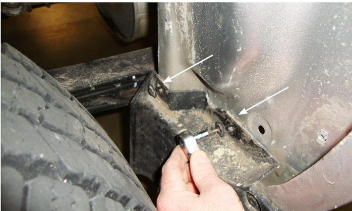
2. Reinstall 2 factory screws that hold the factory rock guard on the front side of the fender and tighten.
