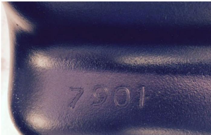
3. Verify that you are installing the correct Wheel Well Guard by checking the part no. located on the backside of the part.
