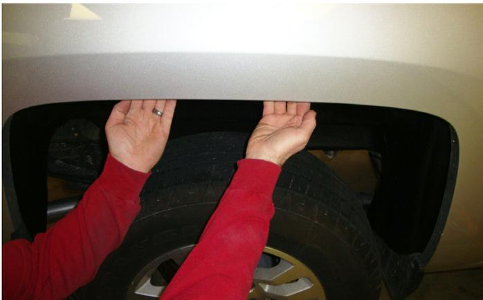
7. Tuck the remaining portion of the Wheel Well Guard behind the fender lip all the way around the fenderwell opening.
