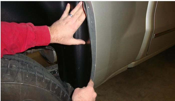
6. Insert the lower flap sections of the Wheel Well Guard into the fender well behind the fender well lip. Perform this step for both the front and rear lower flap sections.
