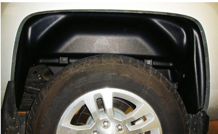
9. Once all fasteners at locations A,B,C & D are installed, tighten with the Torx 15 bit / driver.
