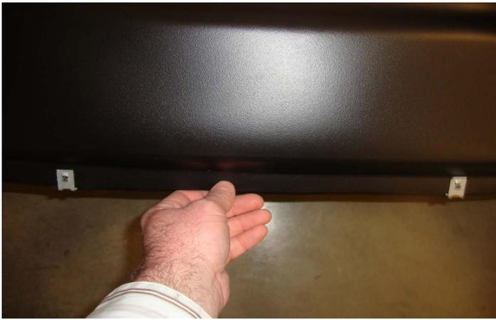
2. Install 2 U-Clips over the Wheel Well Guard's pre-drilled holes at locations B & C.
