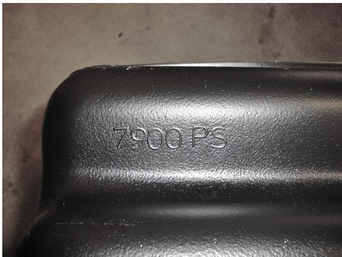
1. Verify that you are installing the correct Wheel Well Guard by checking the part no. located on the backside of the part.
