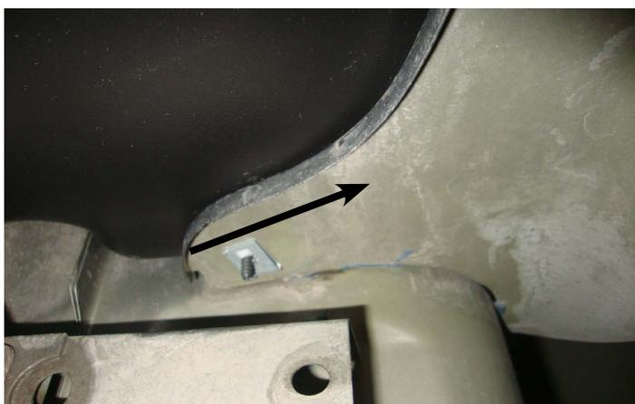
Do not clip the U-clip over the sheet metal. The U-Clip functions as a "nut" and is placed on the backside of the sheet metal.
