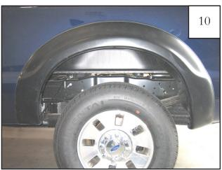
Ensuring that the flare is properly located on fender, tighten all screws.
