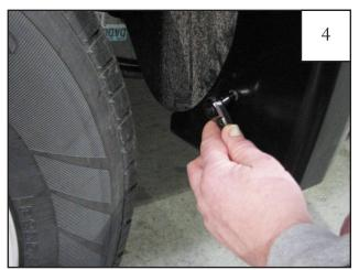
Holding flare in position on fender, reinstall factory screws removed in Step 1.
