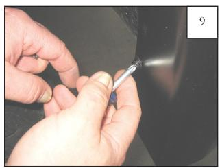
Install five supplied Serrated Flange Screws through remaining holes and into clips installed in Step 8, working from front to back of wheel well.
