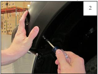
Using a #2 Phillips Screwdriver, install two supplied Plastic Tuf-Loks through additional holes in flare and into fender. *Note: Use a push-twist motion.*
