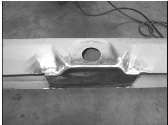
19. Weld backing plate to lower rail flange with two 1/2" long beads at either side. Do NOT add any more weld to bottom of backing plate. Weld top of backing plate as shown to top flange of frame rail. For a cleaner appearance the weld on the top of the backing plate can be ground smooth at this time with a flap disc.
