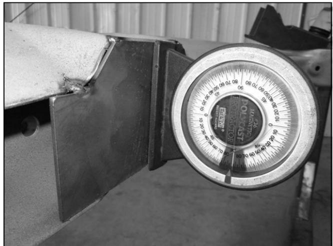
18. Tack backing plate in place as shown with bottom edge of backing plate resting on top of lower rail flange. Make sure that bracket is vertical before proceeding.
