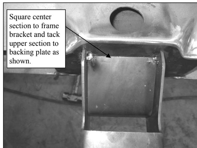
23. The lower plates can now be installed. They can be identified as shown.
