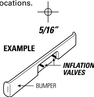
**3** Install Inflation Valve assembly as shown.
