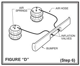
engine, exhaust pipe, and away from sharp edges. Thermal sleeves have been provided for these conditions. The airline tubing should not be bent or curved sharply as it may buckle. Secure the airline tubing in place with the nylon ties provided. Push the end of the airline tubing into the inflation valve as illustrated, **see Figure "E"**.
