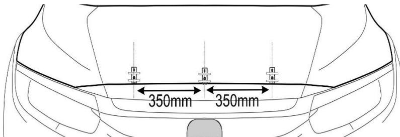
2. The positions of the other pedestals are shown in the illustration. Use the center mark on the leading edge of the pedestals for accurate measuring. The fingers incorporated on the leading edge of the pedestal will help ensure the correct position relative to the hood edge. When correctly positioned the fingers should contact the leading edge of the hood.
