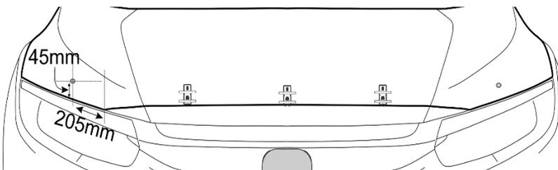
3. Mount the two (2) bumpons in the locations indicated in the illustration. **Note- bumpons must be mounted to the hood surface. If they are mounted to the hood protector they will wear through the paint.**
