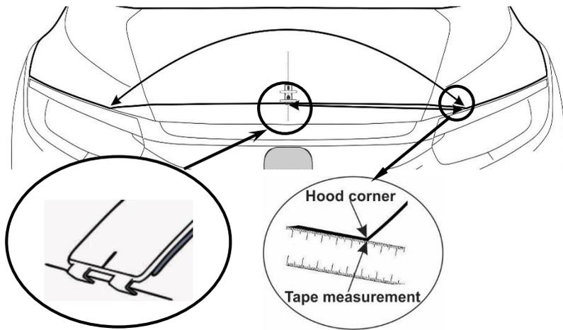
1. Using masking tape or repositionable tape strips supplied, dry-fit an adhesive pedestal at the centre of the hood. To find the center of the leading edge of the hood, use a tape measure to measure to opposite corners of the hood (or some other body line or feature) and adjust the pedestal until both measurements are identical.
