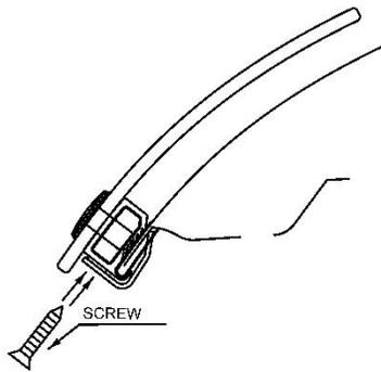
14. Make sure all the components are well seated together and then tighten the screws into the clip bodies.
