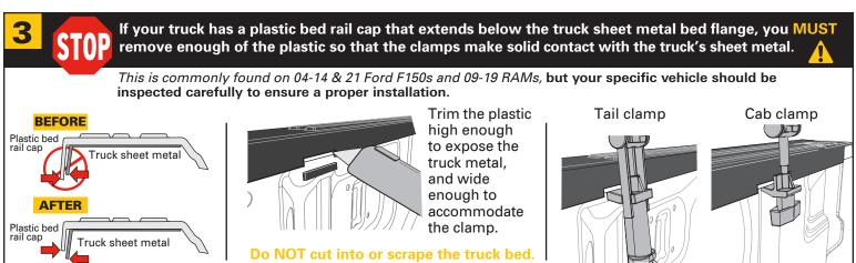
Ensure that the clamp is positioned under the metal bed flange. Hand tighten until clamp contacts the flange, then tighten an additional two turns. Tighten the clamp securely so that the cover does not slide/shift or lift from the truck bed.Do Not secure to only the lip of the bedliner or wall cap. **Do Not Use a Wrench or Overtighten!**
