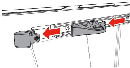
Remove the cargo rail end cap and any tie-down cleats.
