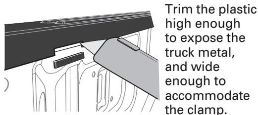
Trim the plastic high enough to expose the truck metal, and wide enough to accommodate the clamp.
