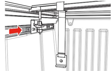
Move the slide block forward to the front bow of the cover.
