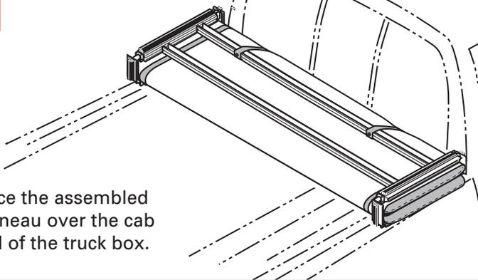
Place the assembled tonneau over the cab end of the truck box.
