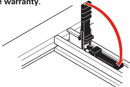
Fold the tonneau forward and fasten the straps in the middle section to the front rail. Check that the straps are tight.
