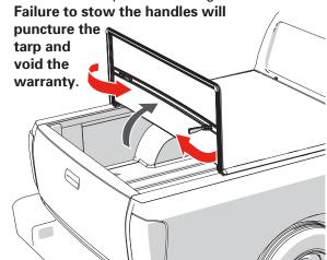
Fold the cover forward and fasten BOTH straps to the front rail. Check that the straps are tight.
