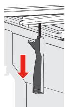
IMPORTANT: Before folding the second section of the cover, the rear clamps must be stowed into the rail to prevent damage to the fabric.
