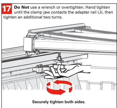
The tethers come installed looped over the bed cover bow with a clamp at the other end. Install the clamp end by sliding the clamp onto the adapter rail (J). Make sure the clamp is positioned as far up onto the rail as possible. Firmly hand tighten the knobs. Install the tethers on both sides of the cover.
