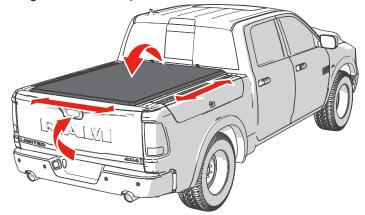
Open the tailgate, swing the tail clamps down from the stowed position and slide them at an angle toward the truck bed rail. Swing the clamps and pull down so the clamp jaw is under the metal truck bed rail flange. Check that both
