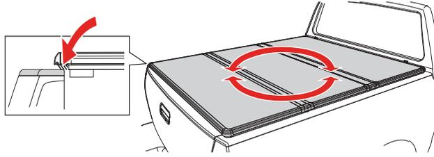
**3** Carefully re-fold the bed cover (A) without shifting its position on the truck bed.
