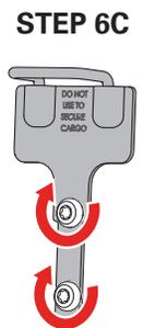
**9** The tethers come installed on the bed cover hinge with a clamp at the other end. Install the clamp end by sliding the clamp onto the truck rail. Make sure the clamp is positioned as far up onto the rail as possible. Firmly hand tighten the knobs. Install the tethers on both sides of the cover.
