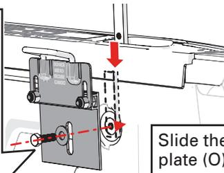
Slide the backing plate (O) up until it contacts the bottom of the bed cap. Tighten the 5/16" -18x1" bolt (M).
