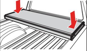
**2** Unfold the bed cover (A) fully and adjust position over the truck bed for proper front (cab) and rear (tailgate) alignment. When positioned front and back, the tailgate seal should contact the tailgate with the first two fins.
