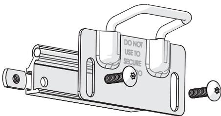
The brackets are assemblies comprised of the striker bracket (C), T-27 Torx screws (B), a backing plate (E) and a weld nut (D).
