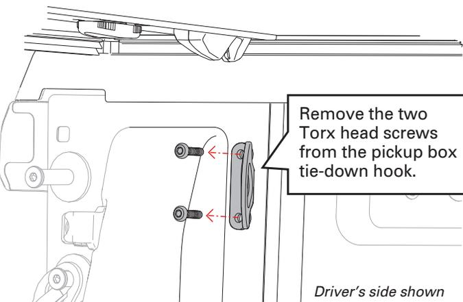
Remove the two Torx head screws from the pickup box tie-down hook.
