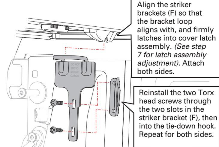
Align the striker brackets (F) so that the bracket loop aligns with, and firmly latches into cover latch assembly. (See step 7 for latch assembly adjustment). Attach both sides.
