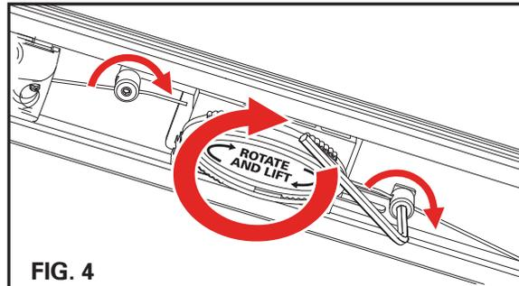
**8** To make the final adjustment, loosen the striker bracket bolts or screws. Then move the bracket (C, F, H, or Q) down by firmly pushing the cover (A) to the truck rail and tailgate. Make sure that both sides match, then retighten all the screws while maintaining the pressure on the cover.
