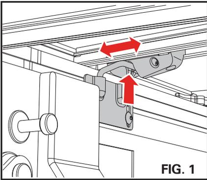
Lower the rear of the bed cover and loosen the screws on both latch assemblies and the rotary knob. Rotate the knob to locate the screws. Adjust the position of each latch so that they engage with the striker brackets, (Fig. 1). With the latches adjusted, from underneath the cover, use the provided T-20 Torx wrench to tighten the two screws, (Fig. 2) in both the driver and passenger side latches.
