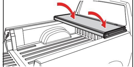
**4** Slide the cab clamps over to the truck bed rail. Align the clamp by rotating until the clamp pad is aligned as shown.
