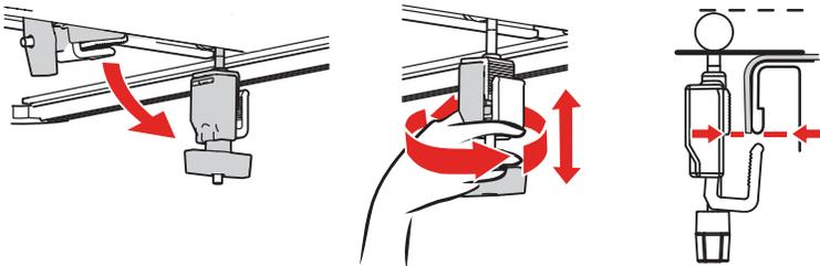
Push the clamp to the truck bed rail, rotate the jaw up under the rail and tighten.
