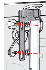
In both cases, the bolts or nuts will be tightened after the final bracket adjustment in step 8.
