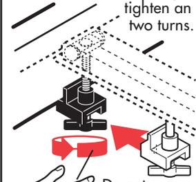
Do not secure to only lip of bedliner or wall cap. Do Not Use Wrench or Overtighten!
