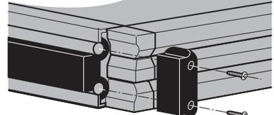
To remove foreign matter from panel hinges, remove one end cap and slide panels apart. Reassemble after cleaning.
