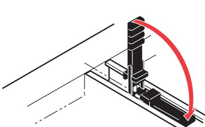
IMPORTANT: Before folding the second section of the cover, rear clamps must be stowed securely into rail.
