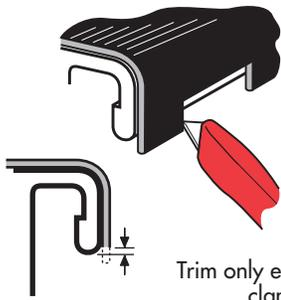
Trim only enough of the bed cap edge or liner wall so clamp contacts bottom of metal flange.
