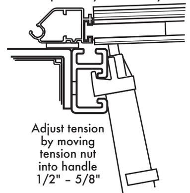
Adjust tension by moving tension nut into handle 1/2" - 5/8"
