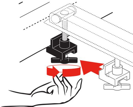
**10** With the tailgate open and the front (cab) clamps secure, completely close the cover
