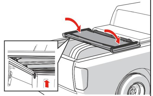
**8** **STOP** If your truck has a plastic bed rail cap that extends below the truck sheet metal bed flange, you **MUST** remove enough of the plastic so that the clamps make solid contact with the truck's sheet metal.
