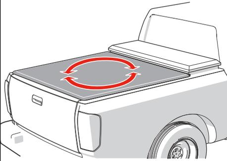
Then carefully re-fold the cover without shifting its position on the truck bed.
