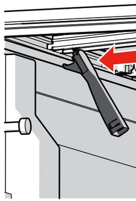
The clamps should be slid, at a slight angle, as far over to the rail as possible.
