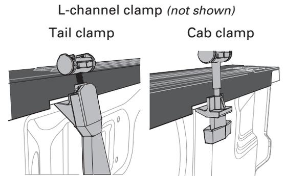
Check all 6 clamps (L-channel, cab and tail) to make sure there is solid contact with the truck's sheet metal after trimming.
