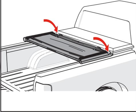
**7** Unfold the cover fully and adjust the position over the truck bed for proper cab and tail alignment. **Note the position of the clamps for the following steps.**
