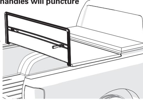
Fold the cover forward and fasten the straps to the front rail. Check that the straps are tight.
