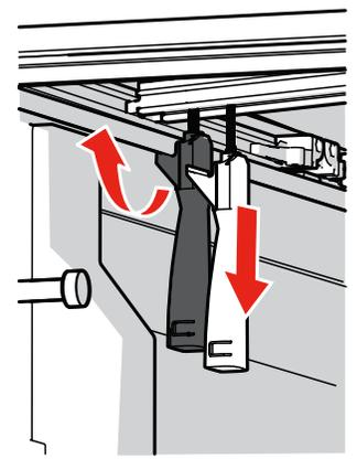
Pull the clamps straight down and release them to hook under the bottom of the metal truck bed rail flange. Always latch the clamps on both sides of the bed.
