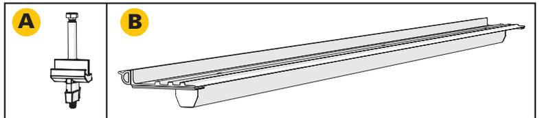
**1** Assemble the L-channel clamp (A) as shown, insert the bolt through the hole in the top of the L-channel rail (B), through the plastic sleeve, through the clamp jaw and threaded into the T-handle from the bottom of L-channel rail (B).
