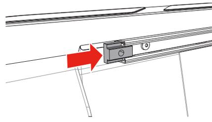
Insert the provided slide block into the cargo rail.
