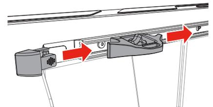
Reinstall any tie-down cleats and the end cap on both sides of the truck.
