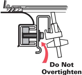
Add the clamp plate, washers and screws as shown.
