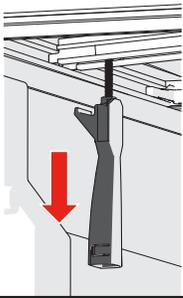
**IMPORTANT:** Before folding the second section of the cover, the rear clamps must be stowed into the rail to prevent damage to the fabric. **Failure to stow the handles will puncture the tarp and void the warranty.**
