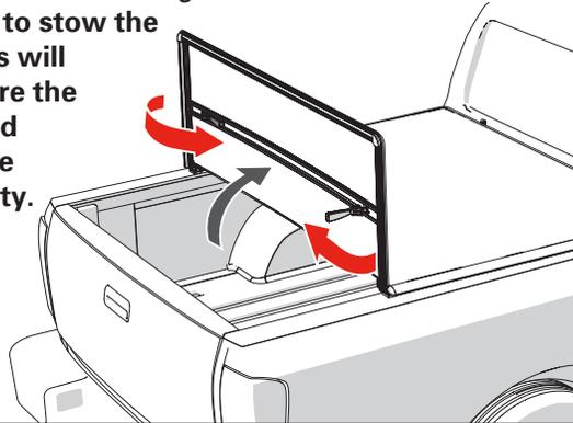
Fold the cover forward and fasten the straps to the front rail. Check that the straps are tight
