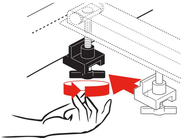
**5** With the tailgate open and the front (cab) clamps secure, completely close the cover
