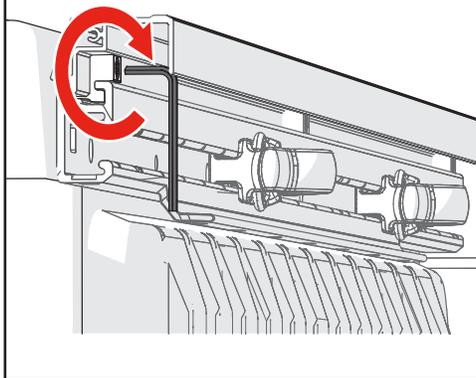
**13** Attach the rail end caps (M) to the adapter rail (H) with the flat rail end cap screws (N).
