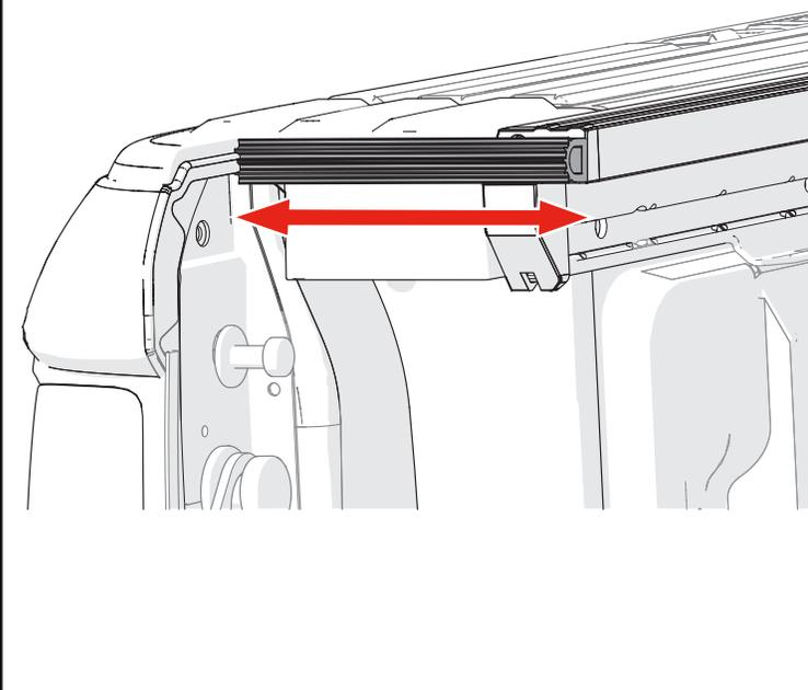
**15** Place the cover (A) onto the truck bed rails and bulkhead. **NOTE:** Take care not to damage or deform the cover seals while installing the cover.
