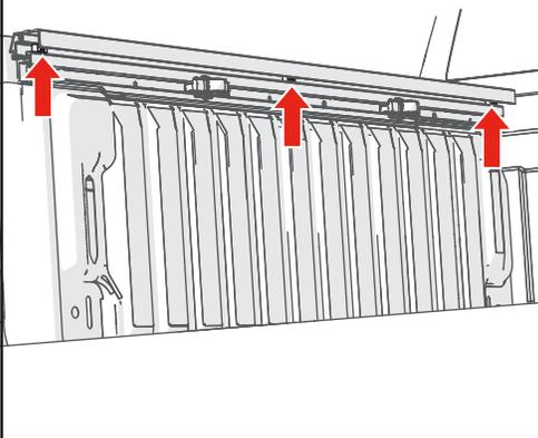
**12** With the adapter rail (H) firmly pressed up to the bulkhead, tighten each lock block (F) with the 3/16" hex wrench provided.
