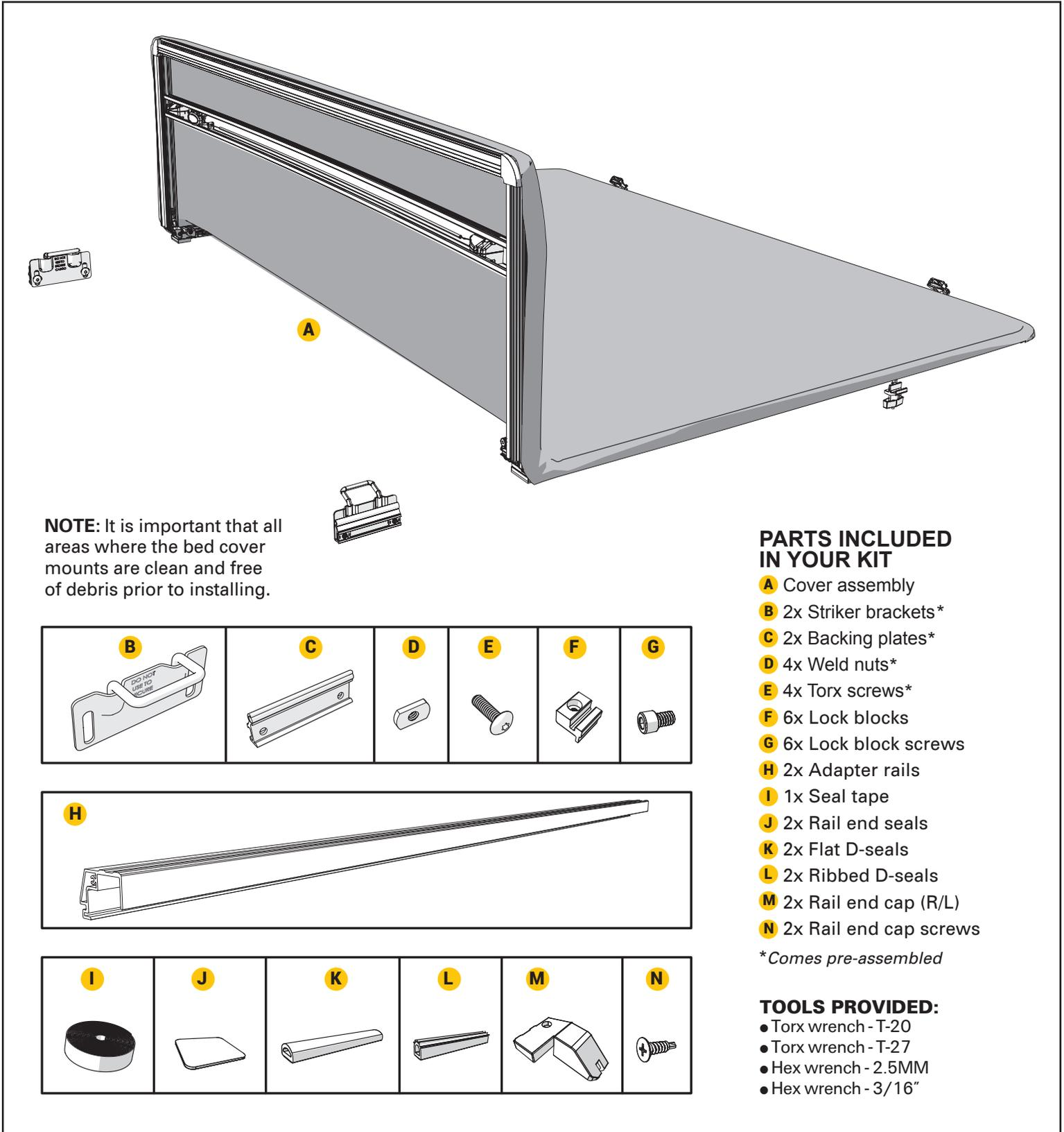
**NOTE:** It is important that all areas where the bed cover mounts are clean and free of debris prior to installing.
