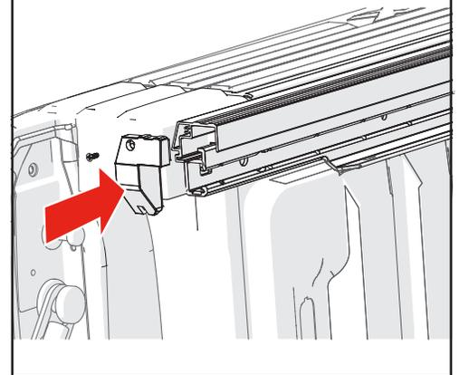
**14** Adhere the ribbed D-seal (L) in the end cap corner to span the adapter rail (H) end cap and rear trim panel. Add one to each side. Trimming the seal may be required.
