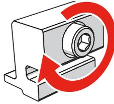
**NOTE:** Keep the screws loose, they will be tightened after they are inserted into the rail.
