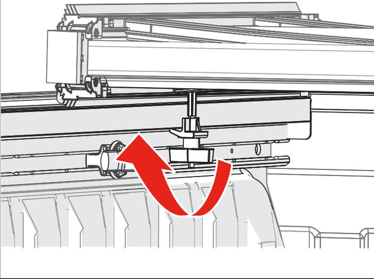
**17** Do Not use a wrench or overtighten. Hand tighten until the clamp jaw contacts the adapter rail (H), then tighten an additional two turns.
