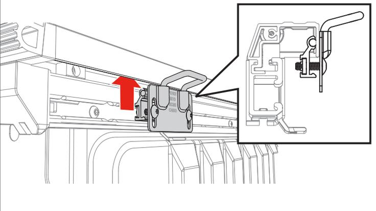
**21** Close the cover (A) and align the striker bracket (B) with the bed cover latch. Push down on the cover while tightening the Torx screws (E).
